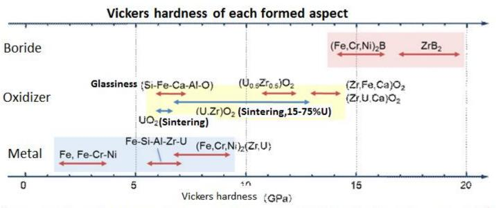
(Estimate hardness distribution for each chemical system of fuel debris (boride, oxide, metal)
