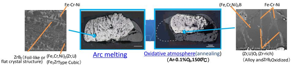
Reaction with control material (B<sub>4</sub>C+SUS) (Example of the fusion solidification abstaining from side observation image
