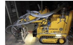
High pressure water jet
