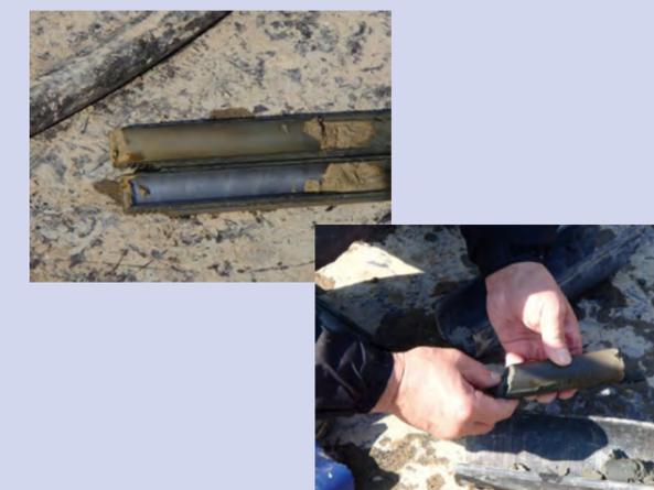
Photo 2 Soil sample taken during boring survey
