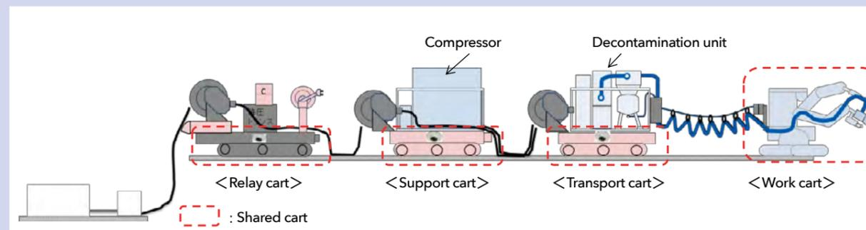
Figure 4 Conceptual diagram of upper floor decontamination equipment (shows mounted blast equipment as an example).
