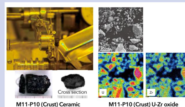
Figure 4 Cutting of TMI-2 debris sample and SEM/EPMA analysis of cutting dust
