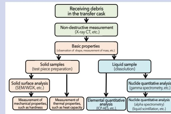
Figure 1 Overall debris analysis workflow plan (outline)
