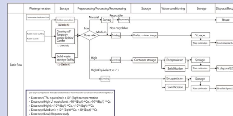
Figure 5 Example of series of handling processes for storage, processing and disposal of waste
