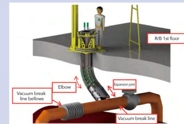
Figure 4 Flexible guide pipe overview
