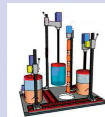
Figure 3 Shield plug hole boring device (image)
