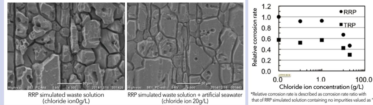
(1) Surface observations of immersion test piece
