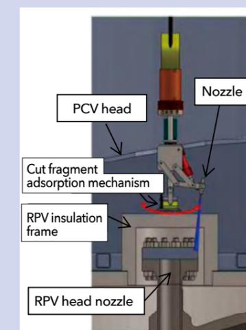
Figure 4 RPV head hole boring device (image)
