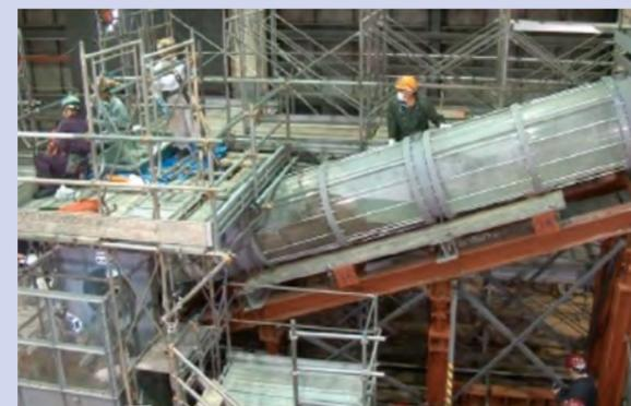
Figure 3 Water stoppage testing using a one-half model of the bent pipe
