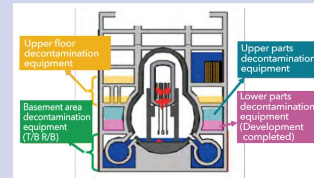
Figure 1 Locations where each type of decontamination equipment is to be placed.
