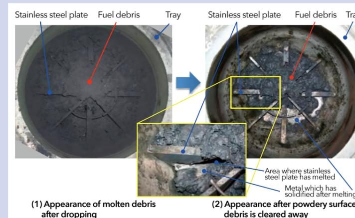
Figure 3 Result of fabrication of metal and ceramic solidified products produced at the Kazakhstan National Nuclear Energy Center (NNC)
