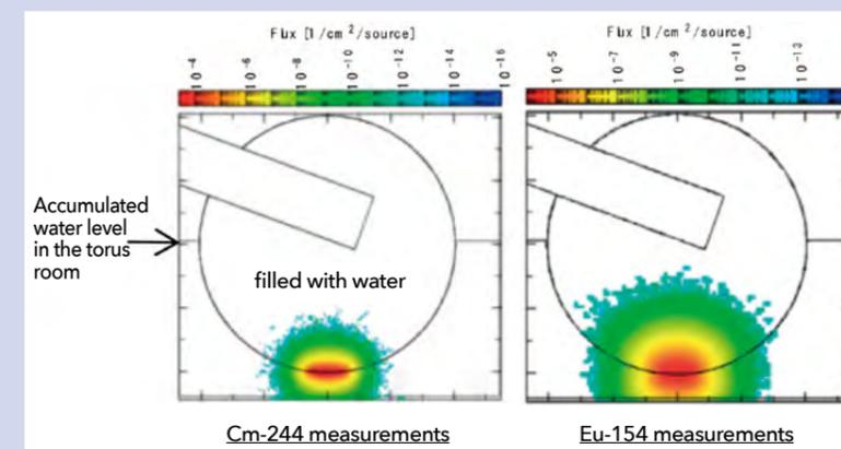
Figure 2 Distribution of radiation originating from fuel in the vicinity of the S/C (Unit 1)
