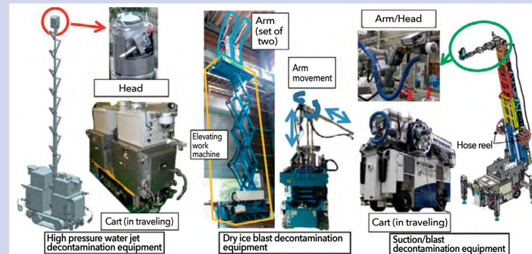
Figure 2 Improvements to equipment for decontamination of upper parts conducted during FY2014.
