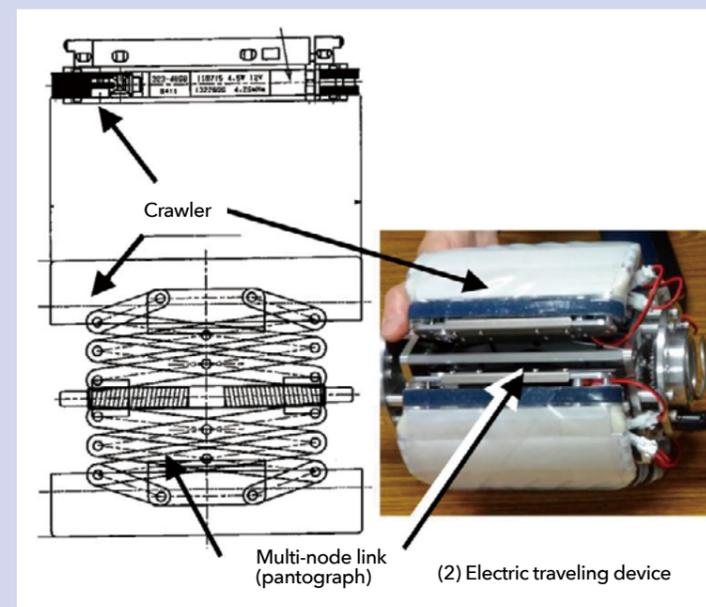
Figure 2 Electric traveling device
