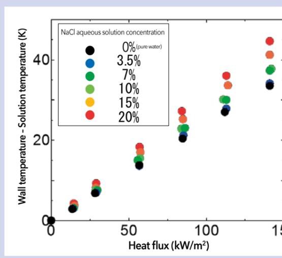
Figure 4 Example of test results using sodium chloride solution (Temperature difference between wall and solution)
