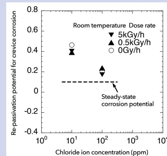
Figure 4 Relationship diagram between re-passivation potential for crevice corrosion in diluted artificial seawater and chloride ion concentration obtained through electrochemical test using crevice corrosion test specimen (testing using crevice corrosion specimen made of a combination of Zr and SUS304L).
