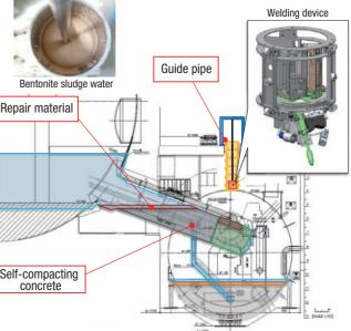
Vent pipe 1/1 scale test
