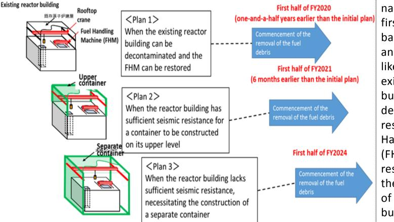
\*Future plans will be narrowed down in the first half of FY2014 based on the results of analysis of the likelihood of the existing reactor building's decontamination or restoration of the Fuel Handing Machine (FHM), as well as the results of assessment of the seismic resistance of the existing reactor building.
