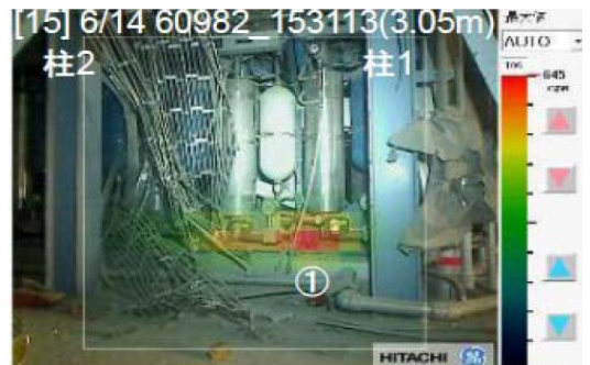
Radiation source survey (gamma camera) results example (Unit 3 South side HCU)
