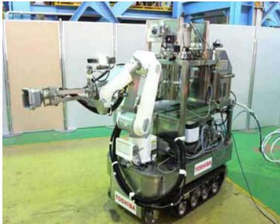
Dry ice blast decontamination device
