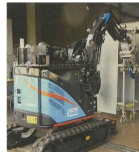
Remote-controlled heavy machinery (ASTACO-SoRa)
