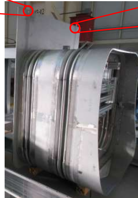
Making the cell adapter guide pin hole
