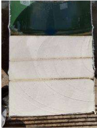
Test No. 7 (3 rounds of injection) cut surface
