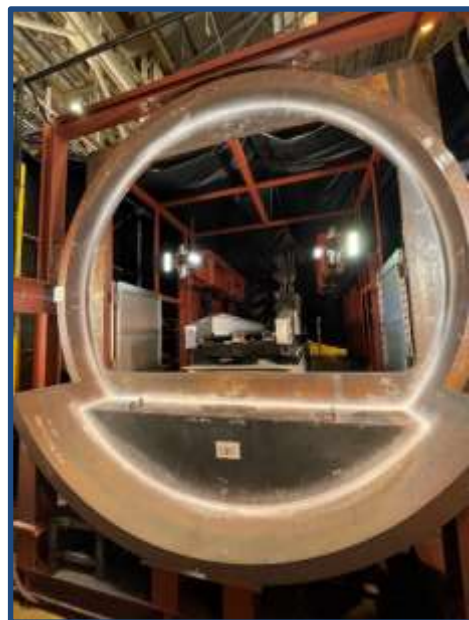
① Dye PT conducted after all-around welding
