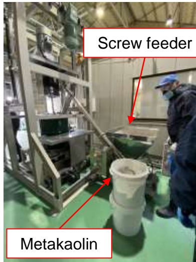
Blending equipment (Pouring Metakaolin)
