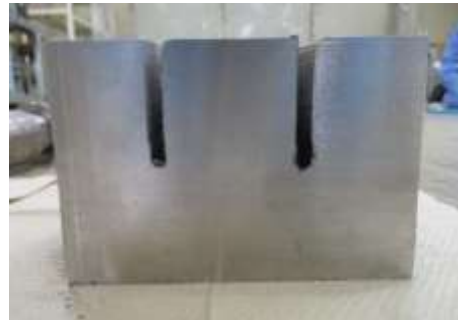
Core boring swarf dischargeability verification test (10kN, 250rpm)
