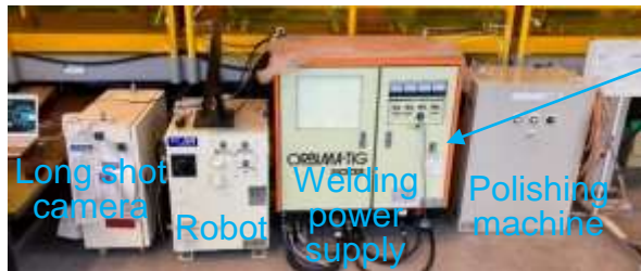
Control equipment (robot, polishing machine, long shot camera) & welding power supply
