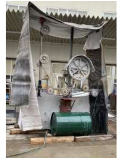
Cutting equipment (Wire saw)
