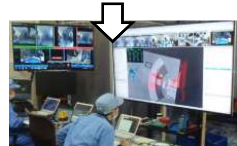
Operation of the actual equipment (site) Each operator operating the actual equipment on site using the trajectory data created during advance planning
