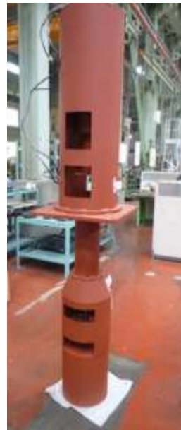
Simulated pump for the element tests
