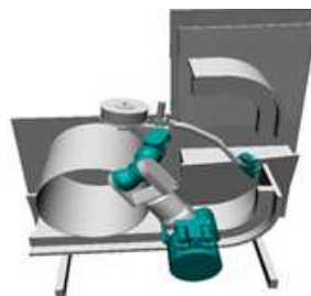
Planning for movement over the welding route (FY2017-FY2018)
