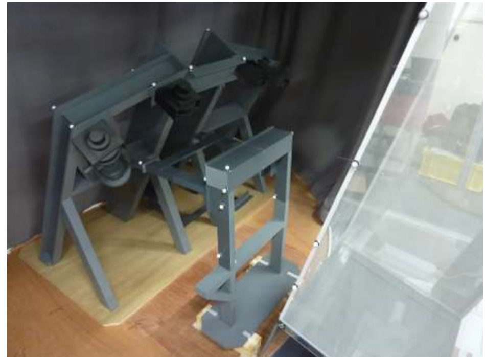
Mock-up of the damaged structures inside the pedestal (A tilted platform frame is present in the vicinity of the opening)
