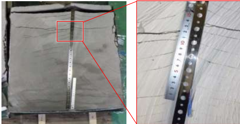
Overall Enlarged view Test No. 1 (Without heating) cross-section Comparison of the cracks and the thermocouple support fittings
