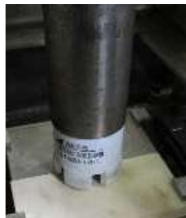
Core boring swarf dischargeability verification test (10kN, 250rpm)
