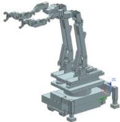
Overview of HVH disassembling robot
