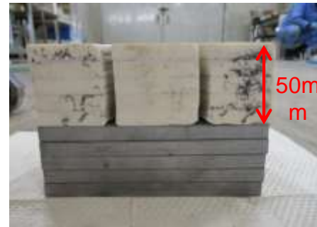
Core boring swarf dischargeability verification test (10kN, 250rpm)
