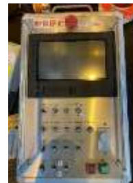
Remote control for the welding operation
