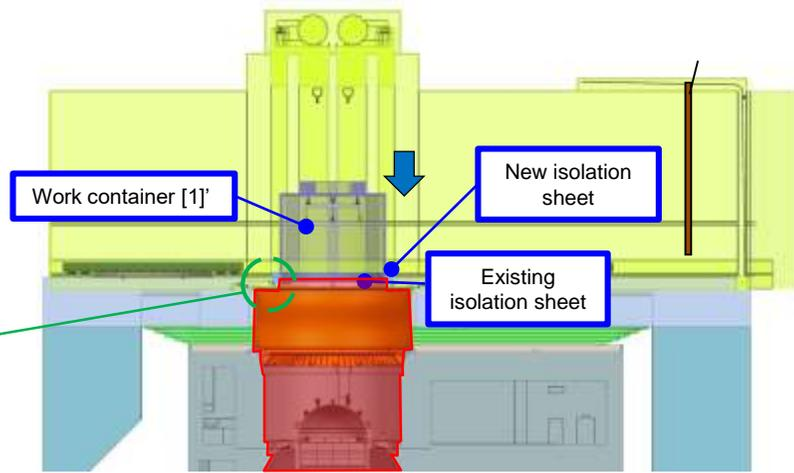
Step 4. Lower the work container, install a new isolation sheet
