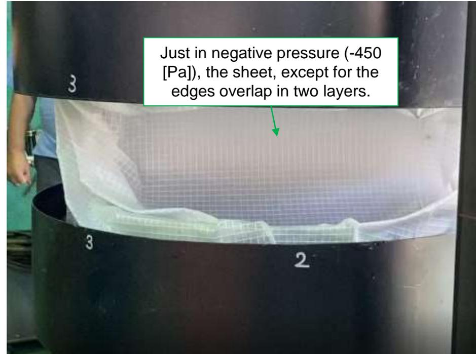
Just in negative pressure (-450 [Pa]), the sheet, except for the edges overlap in two layers.
