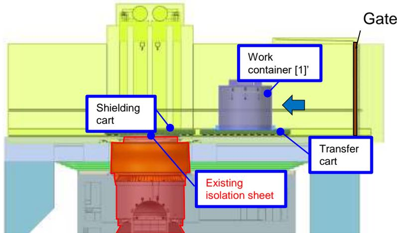
Step 1. Transfer in the work container for structure transfer
