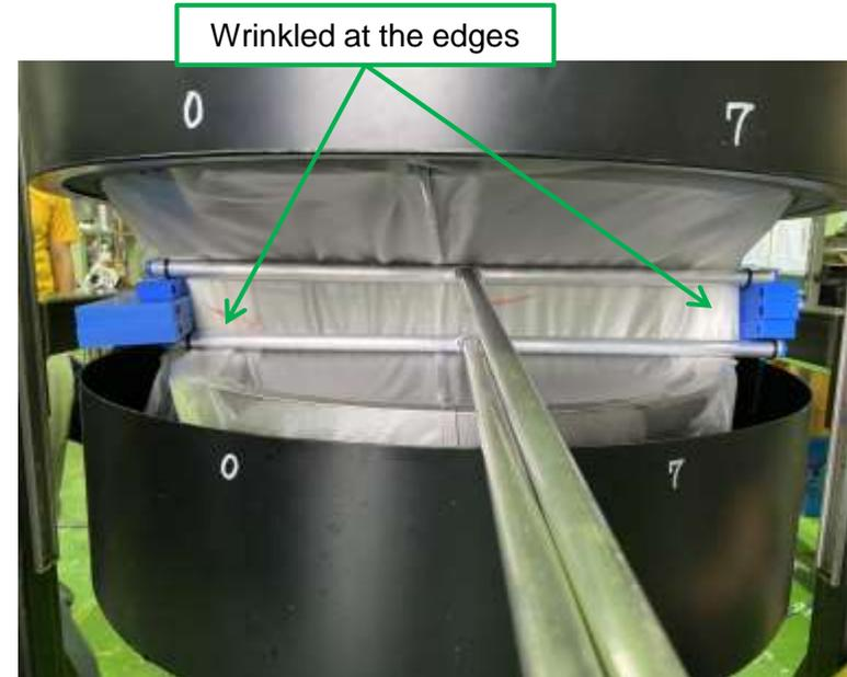
The drum can was fixed and the isolation sheet was manually pulled out and folded
