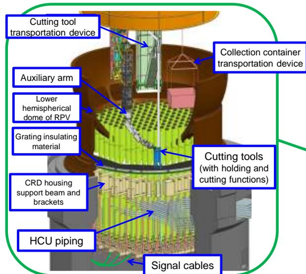
Image of reactor bottom interference objects removal work
