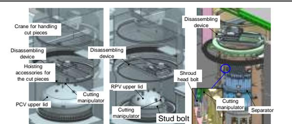
A conceptual study was conducted in the "Development of Technology for Further Increasing the Retrieval Scale of Fuel Debris" (implemented in FY2019-20)
