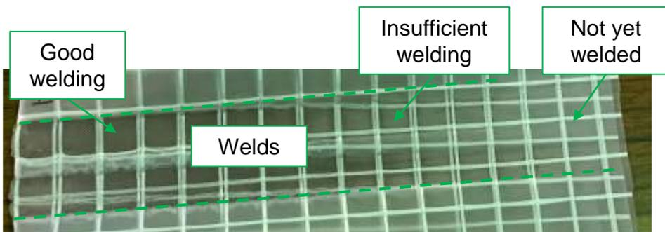
Example of insufficient welding
