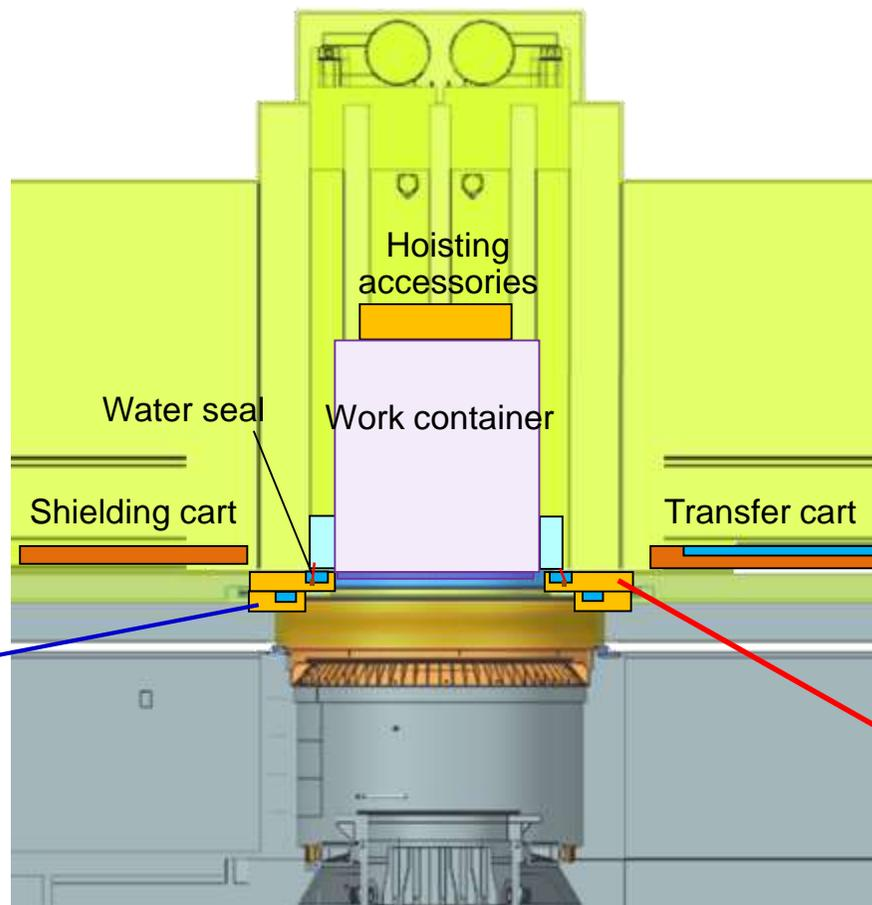
Isolation sheet base for removing structures inside the reactor well (isolation sheet base used when placing the work container on the operation floor and removing the structures in the reactor well)
