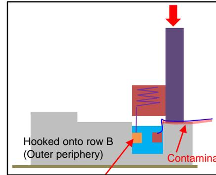
Install a seat on the water seal wall (outer periphery) for hooking on the sheet
