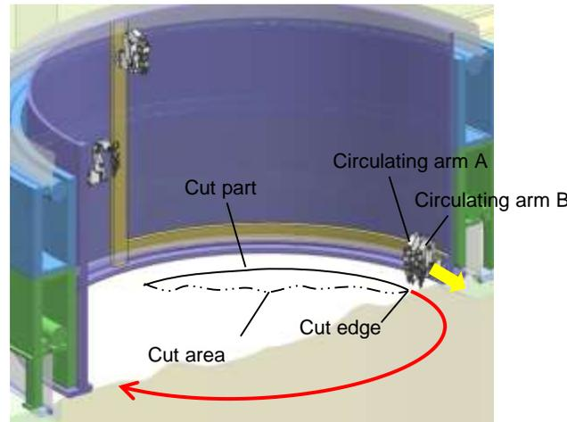
② Grab the cut edge with the circulating arm A and cut the 180° range with the circulating arm B
