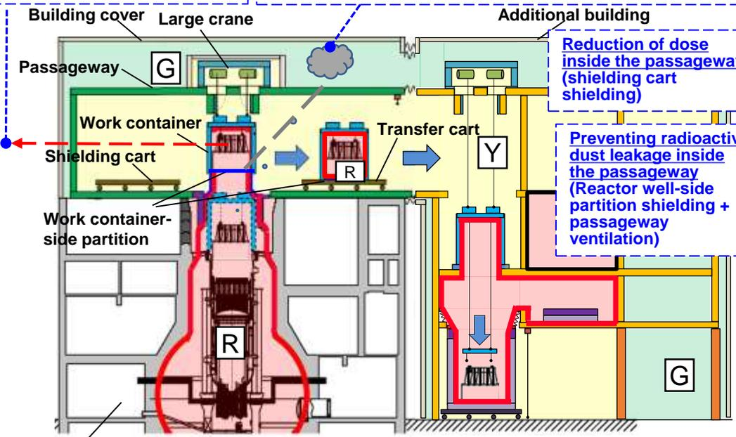
Reactor building During fuel debris retrieval work
