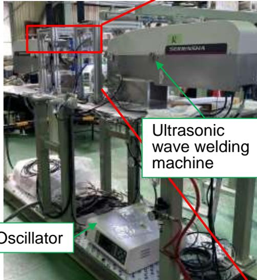
Welding testing device
