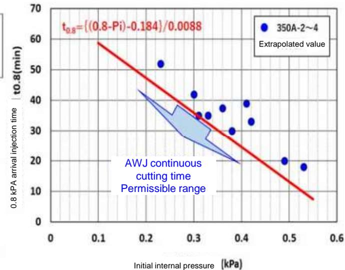
Diagram-2 Relationship between the initial internal pressure and the 0.8 kPa arrival time
