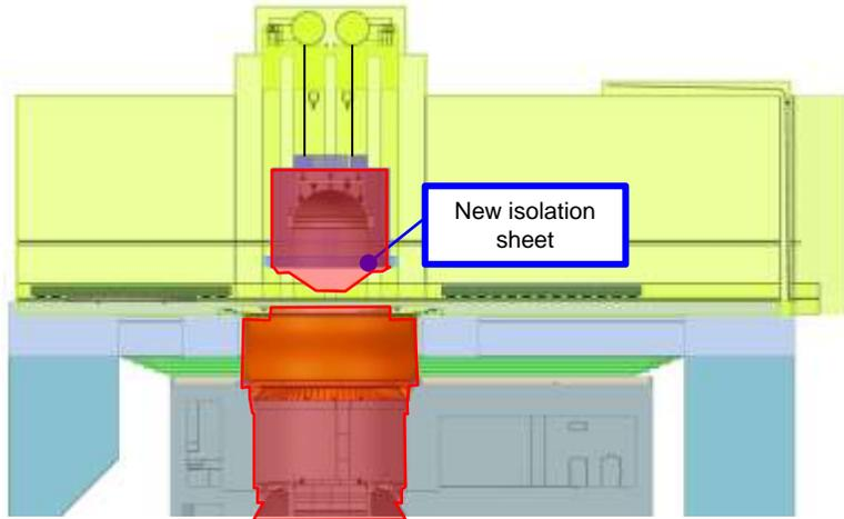
Step 8. Fold, weld, and cut the new isolation sheet (state after cutting)
