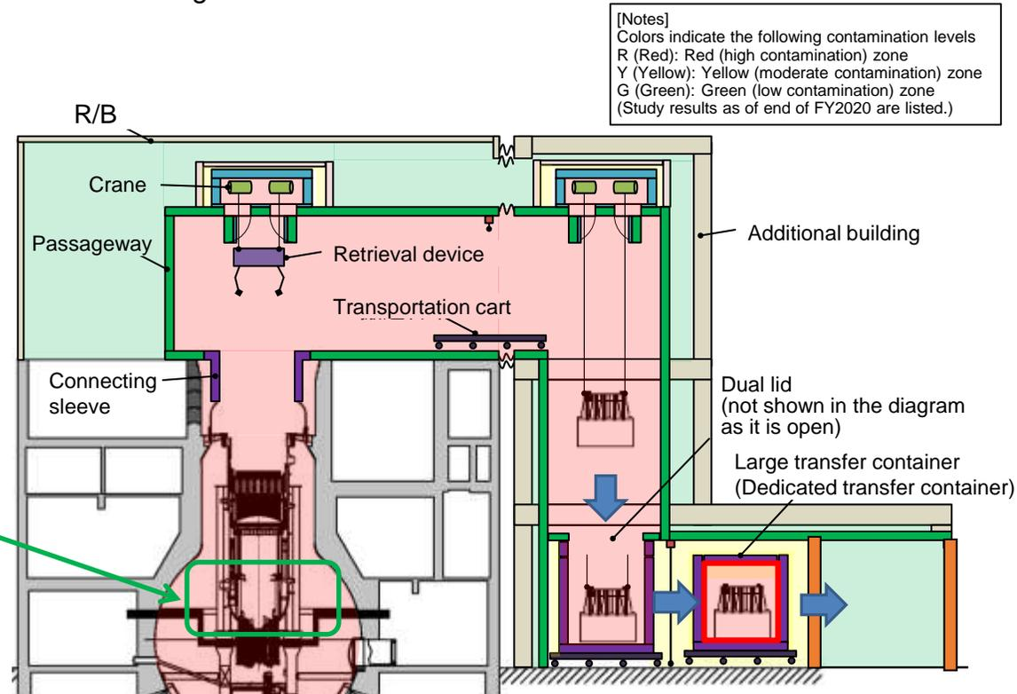
Method for transferring (transfer route) the unitized structure under consideration
