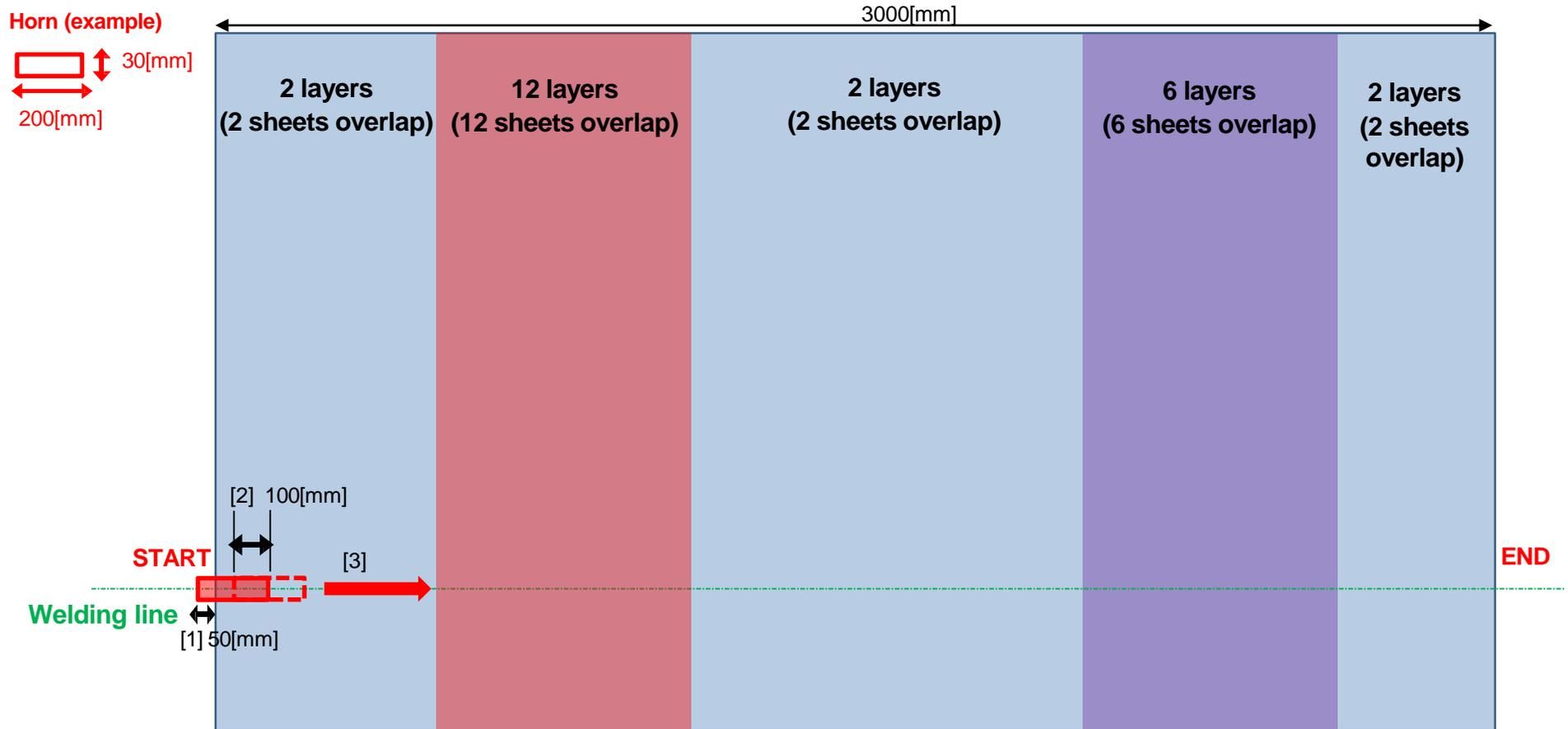
[1] Starts with the horn sticking out of the sheet by 50 [mm]
