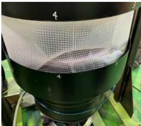
[5] Install the sheet in the water seal in the lower drum can
