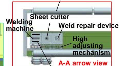
Sheet fixing jig (for welding)
