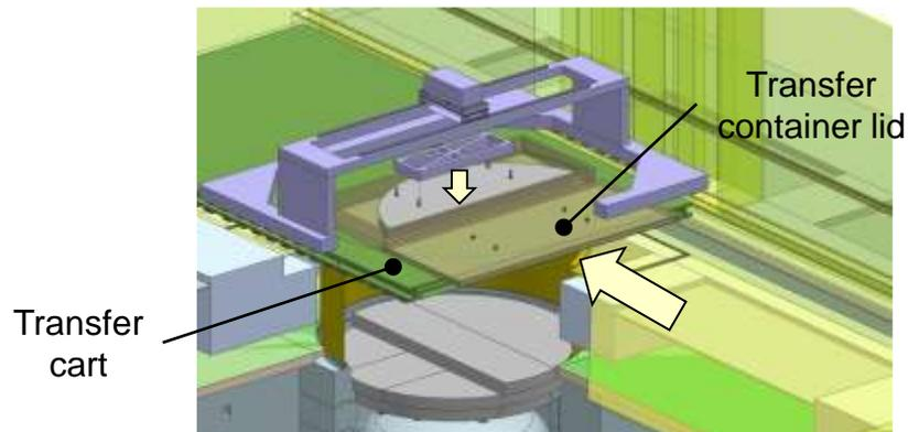
3. Transport the transfer cart to below the shield plug, collect in container
