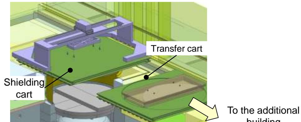
4. Close the transfer container lid, move out the transfer cart
