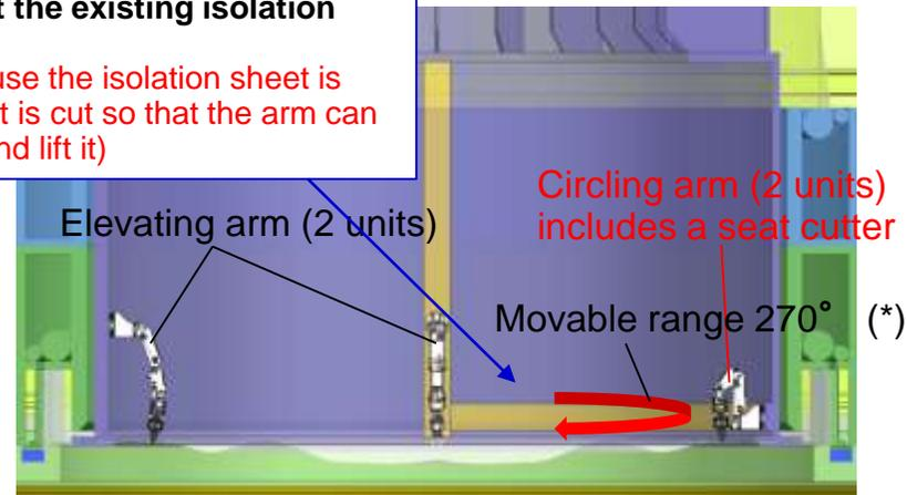
(\*)The remaining 90° of the movable range exists to ensure the sheet is not cut off.
