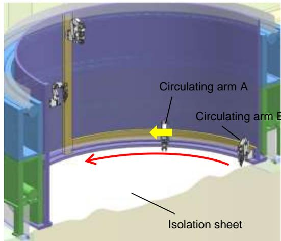
① Grab the sheet with the circulating arm B and cut the 90° range with the circulating arm A
