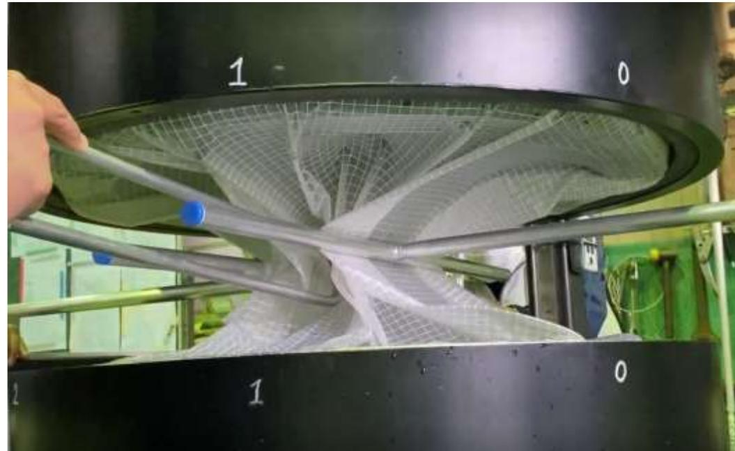
Fold the sheet using the pushing jig together with the fork
