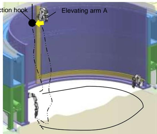
⑥ Hook the sheet held by the elevating arm A onto the collection hook
