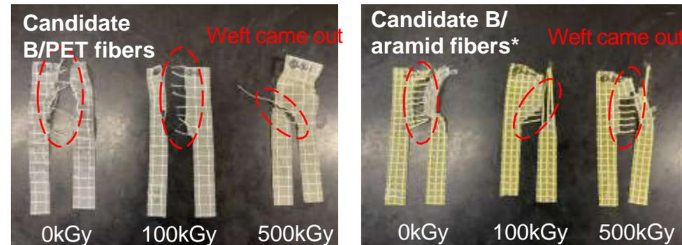
Measuring the tear strength of the sheet with fibers
