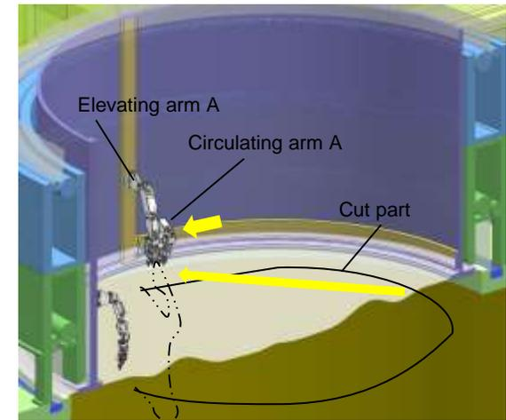
③ Move the circulating arm A near the elevating arm and hand over the sheet to the elevating arm
