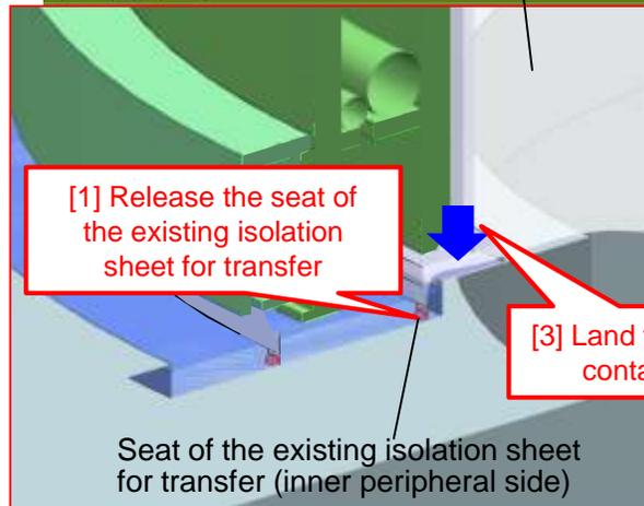
Removed isolation sheet that was attached to the bottom of the container and the existing isolation sheet for transfer
