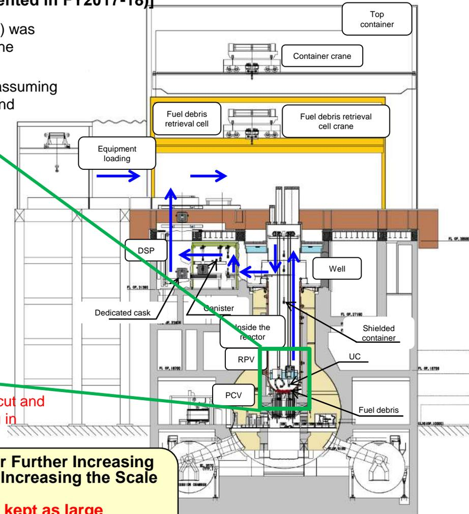
The method for removing large components where structures inside the PCV are cut and stored in unit canisters to be transported outside of the reactor is quite challenging in terms of workability and the time required for work.
