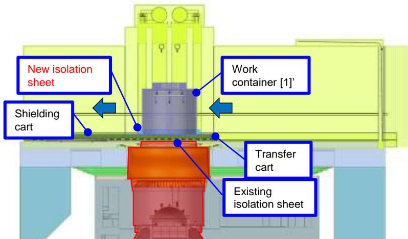
Step 2. Transfer the work container and the shielding cart
