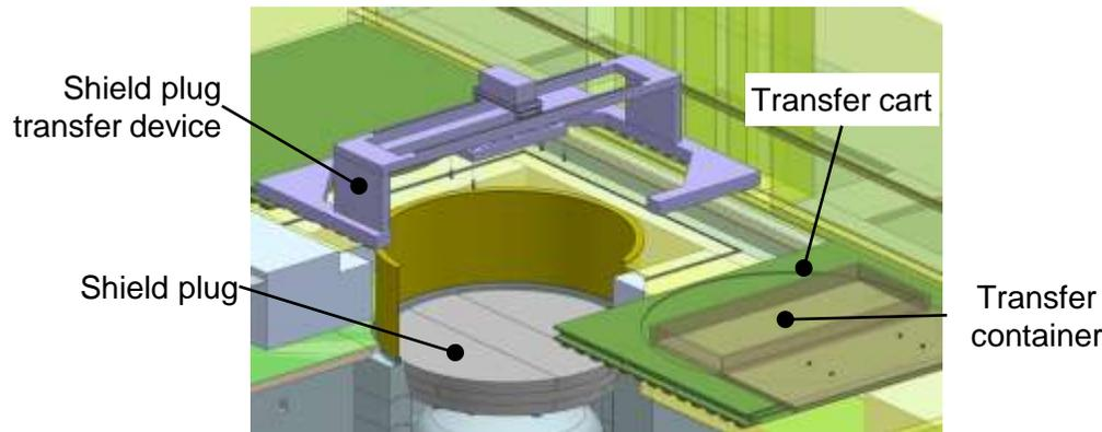
1. Transfer the shield plug transfer device
