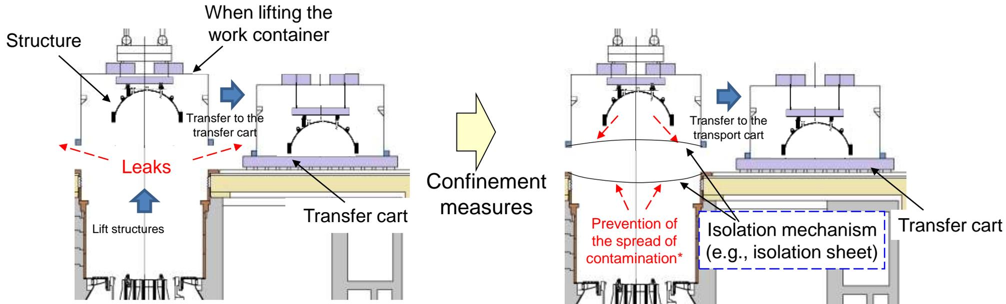
Because the underside of the work container is not closed, it is temporarily open when it is being transferred to the transport cart
