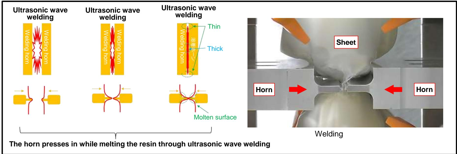
• Insufficient welding occurred in the center where the sheet was thick and defective welding occurred in the thin edges.
