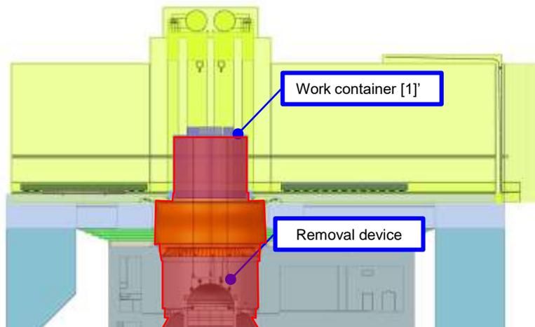
Step 5. Cut the existing isolation sheet, lower the removal device
