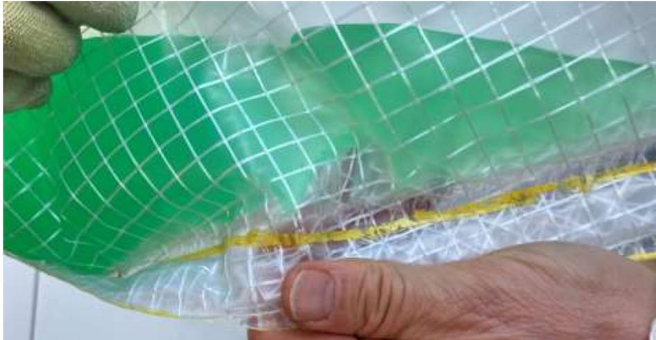
Welding using welding conditions before revision
