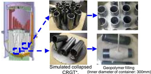
Elemental tests were conducted in "Development of Technology for Further Increasing the Retrieval Scale of Fuel Debris" (FY2019-20)
