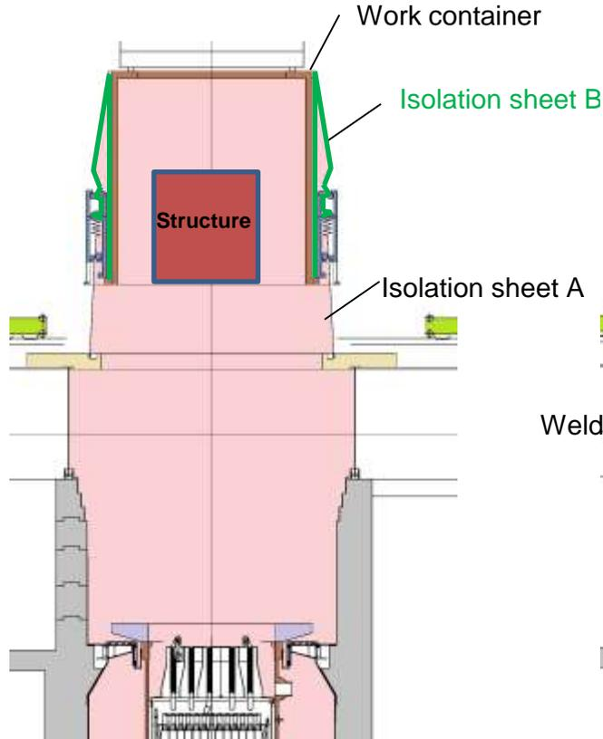
5. Weld and cut isolation sheet A
