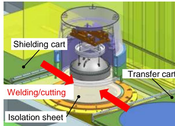
Step 2: Weld and cut the isolation sheet
