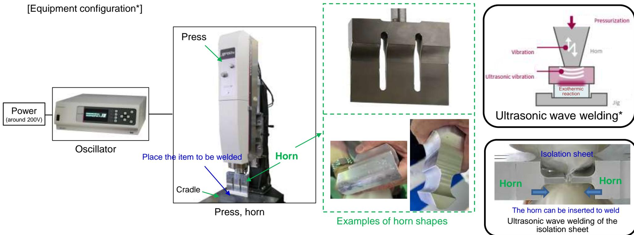
•By adding ultrasonic wave vibrations with the vibrator and pressure to the thermoplastic resin at the same time, the resin can be instantaneously melted and welded.
