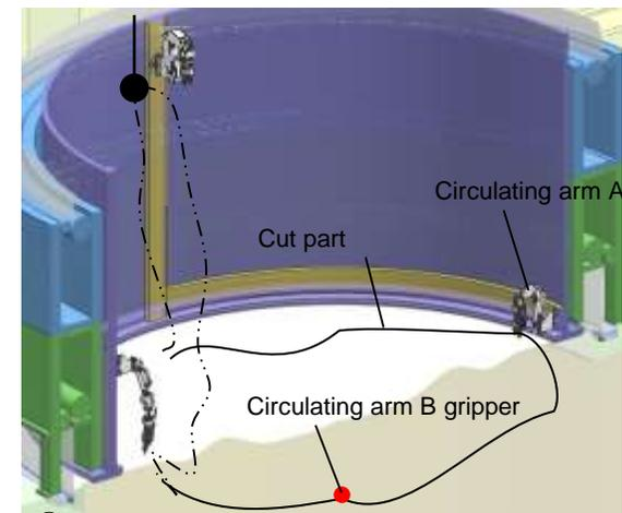
⑦ Hold the remaining part of the cut sheet with the circulating arms A and B (prevent it from falling when the work container is raised)
