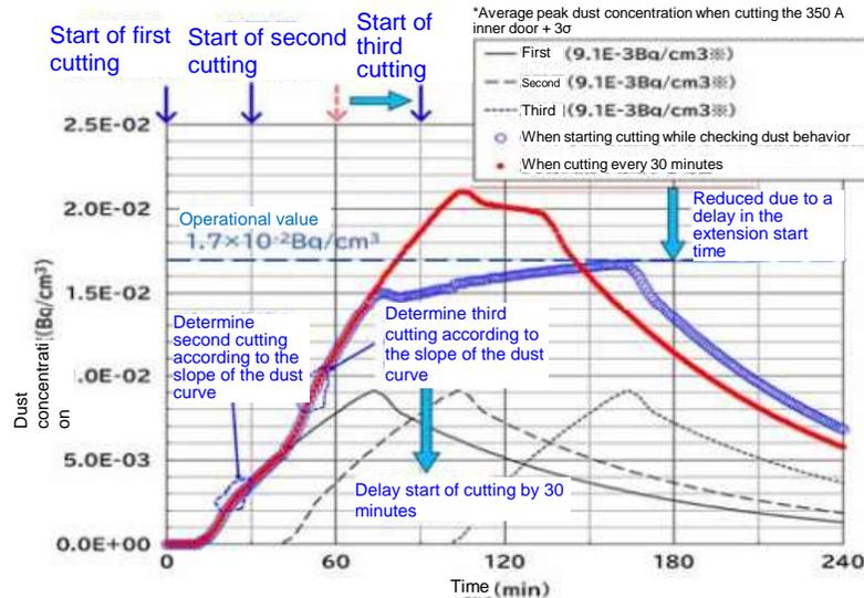
Diagram-1 Method for setting the following cutting start time according to the increases in dust concentration
