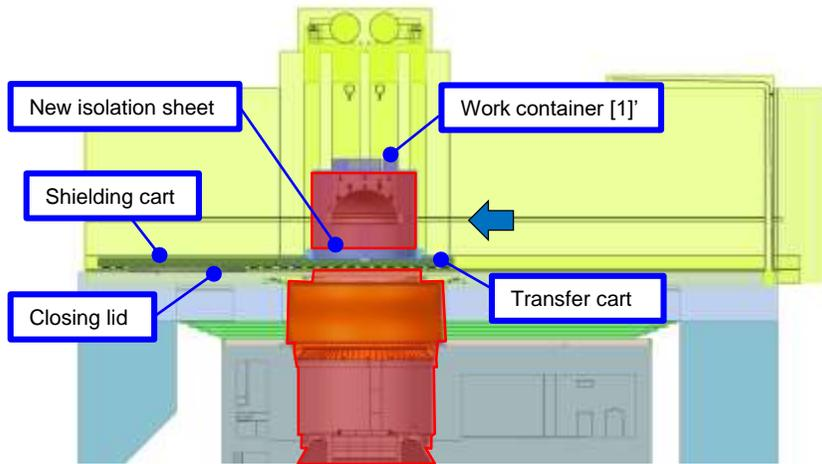
Step 9. Move the transfer car, lift up the work container
