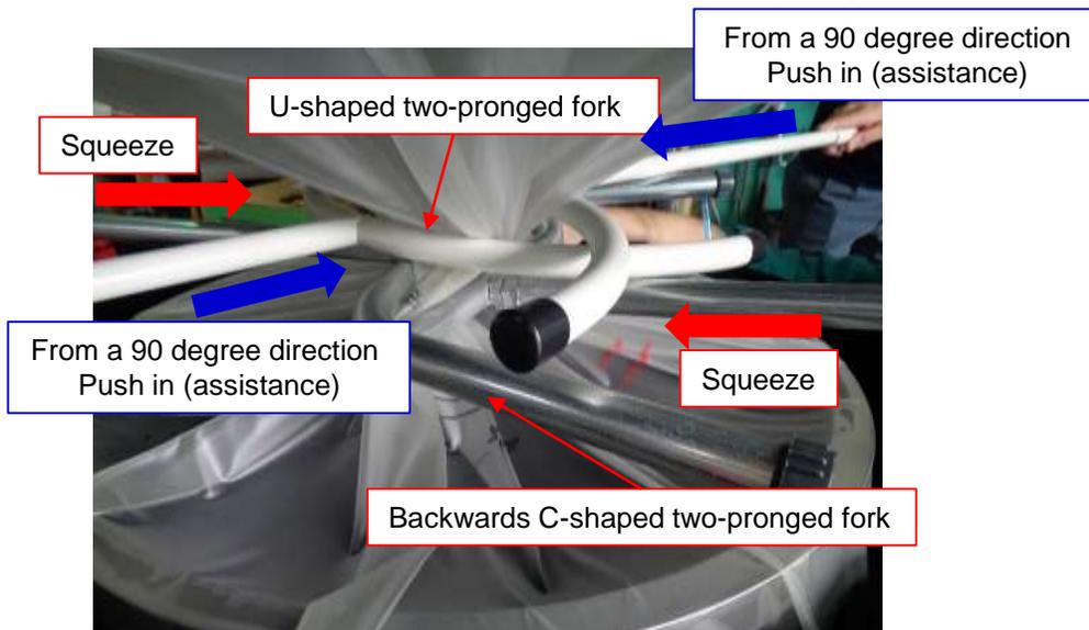
Squeezed with two backward C-shaped two-pronged forks, with two U-shaped two-pronged forks assisting
