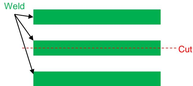
In the current plan, the upper, mid-level and lower lines will be welded and the sheet will be cut at the middle welding line center.
