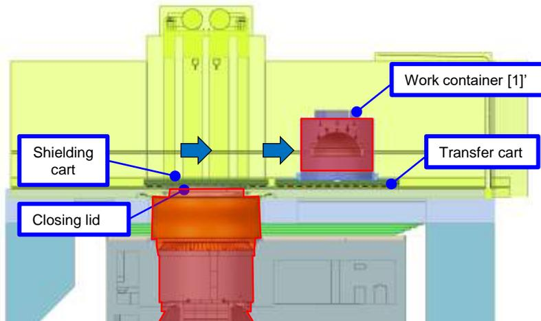
Step 10. Transport the work container, move the shielding cart
