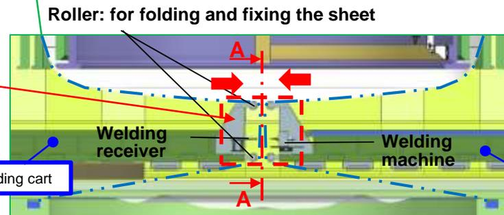
Folding, welding, and cutting the isolation sheet (load the welding machine onto the cart, fold and fix the sheet with the rollers on the top and bottom of the cart, have the welding machine slide in toward the center to weld)
