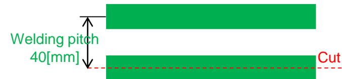
In this test, the two are welded at a welding pitch of 40 [mm] and it is cut at the center of the lower weld line.
