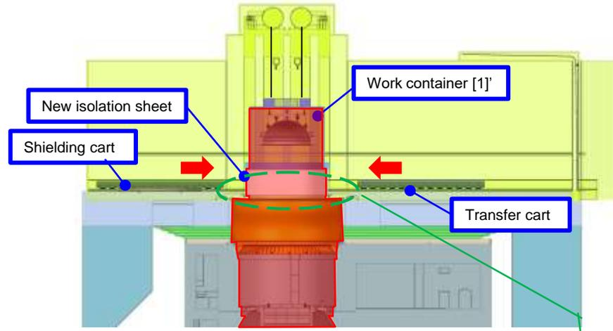
Step 8. Fold, weld, and cut the new isolation sheet
