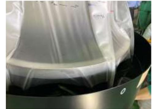
After 10 minutes the clearance for the upper and lower drum cans was 400 [mm] and the differential pressure 450 [Pa]
