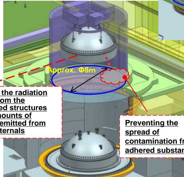
**Shielding the radiation emitted from the transported structures (Large amounts of radiation emitted from reactor internals)**
