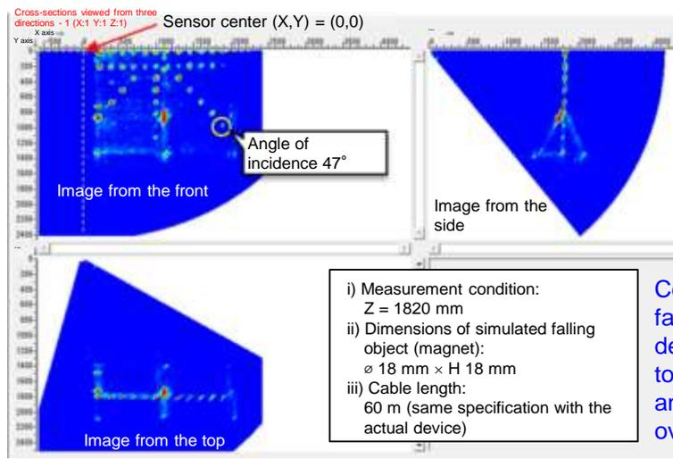
(a) Unit test 1: Verification of measurement pitch
