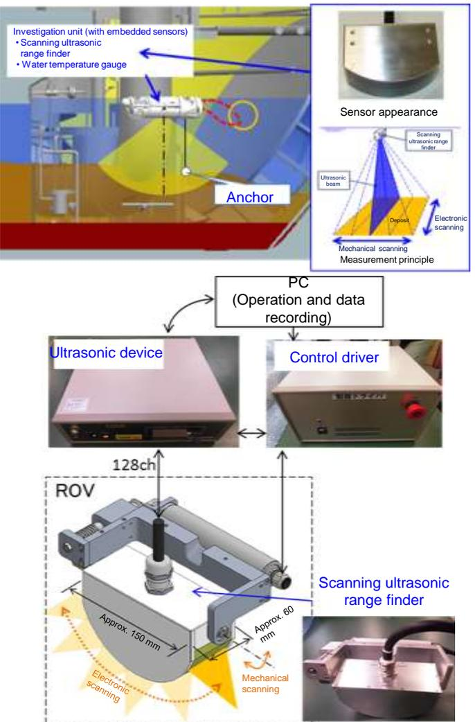
Figure 4.5(1)(ii)-1 Configuration of 3D mapping system
