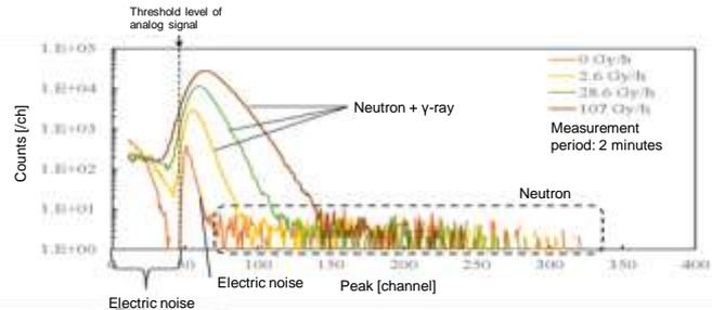
(b) Example of unit test results for B-10 detector
