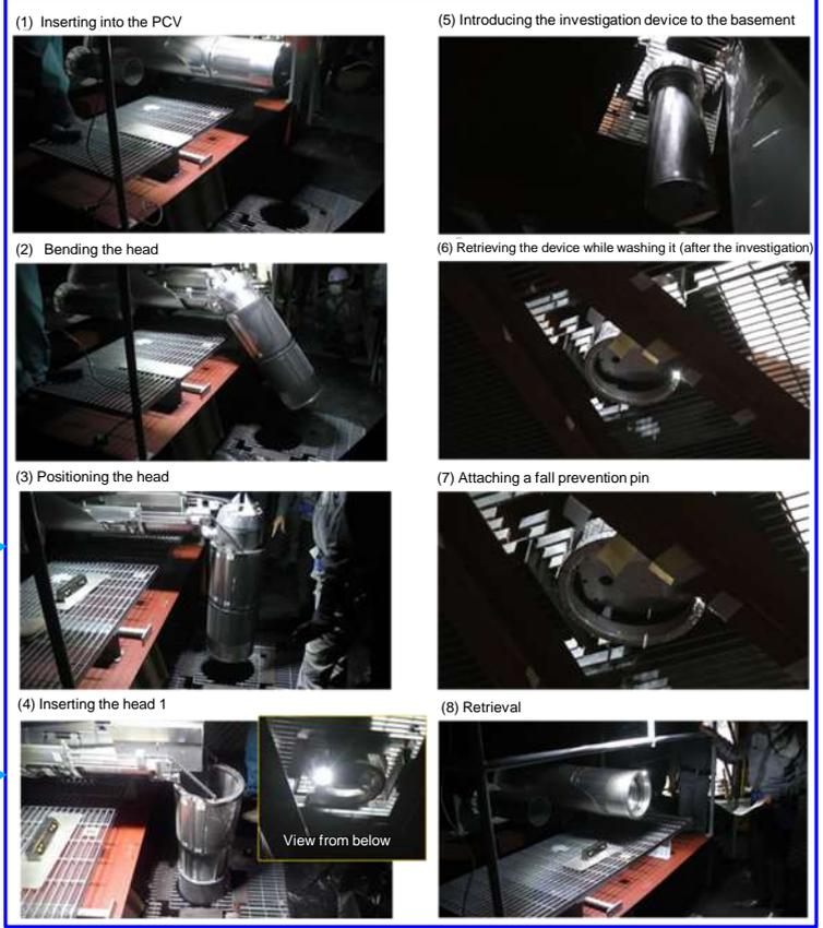
Figure 4.4(3)-1 Illustrations and photos of in-plant verification tests of installation device
