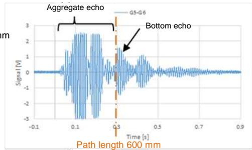
Test results using concrete specimen
