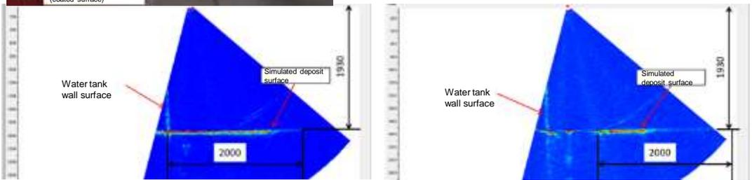
(b) Unit test 2: Detection range for deposit
