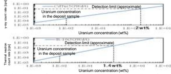
Variation of count rate with the concentration of uranium in the 90-cm-thick deposit
