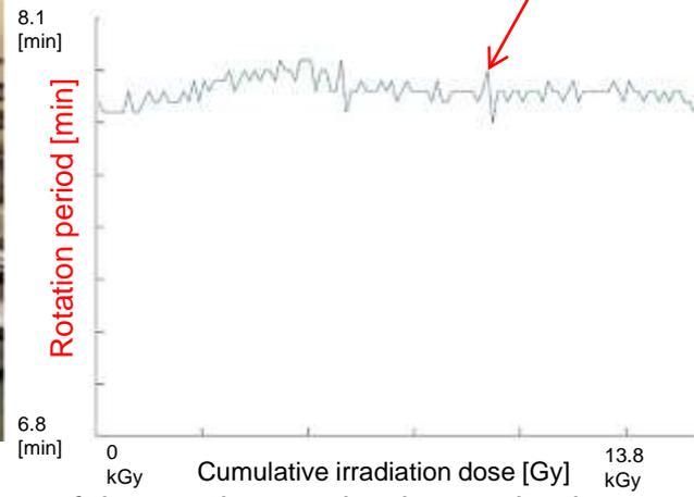
Operational characteristics test of the rotation mechanism under the radiation environment
