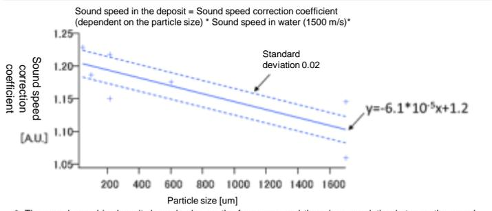
\*: The sound speed in deposit depends also on the frequency, and there is a correlation between the sound speed correction coefficient and the standardized particle size (particle size/wavelength).
