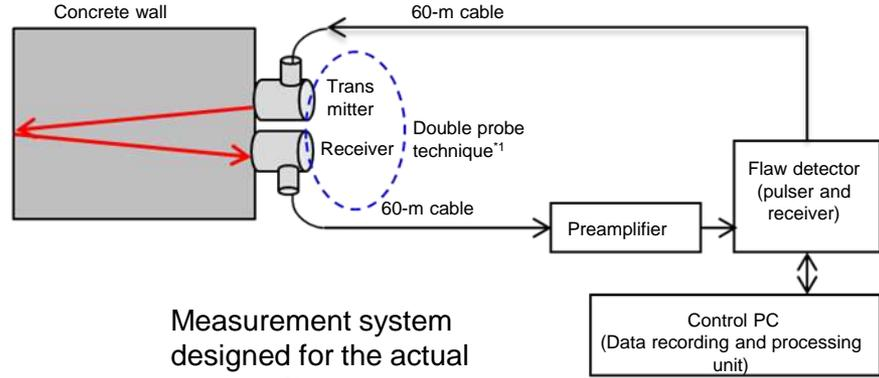
Measurement system designed for the actual device (Plan)
