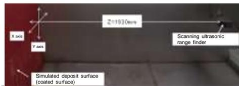
Confirmed that the simulated deposit was visually observed within the range of up to the incidence angle of  $50^\circ$  (beam path length of approx. 3 m)
