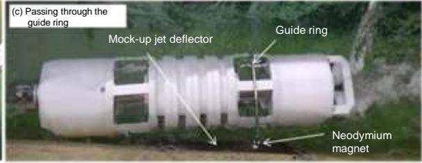
(c) Steps for installing the guide rings
