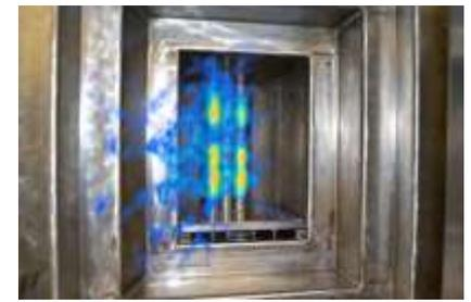
Based on the test measurement data at 1000 Gy/h, the image was converted to the dose data distinguished by irradiation direction. By overlapping it with the image of the actual environment, it was confirmed that the source locations could be identified. (The same test was also performed at 1 Gy/h.)
