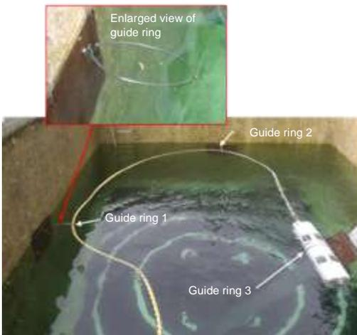
(b) Photos of the guide ring installation test
