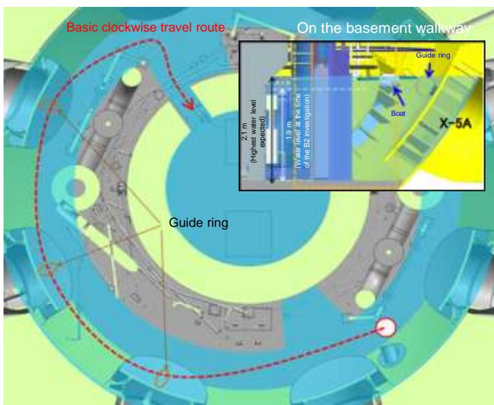
A. Illustration of traveling method in the broad basement area
