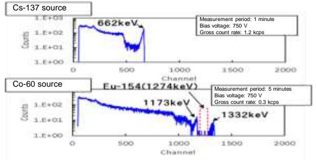
(a) Example of unit test results for CdTe semiconductor detector
