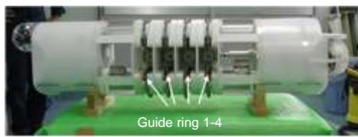
(a) Prototype boat for installing the guide rings
