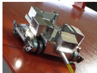
⑥ Exterior surface survey equipment for lower part of S/C
