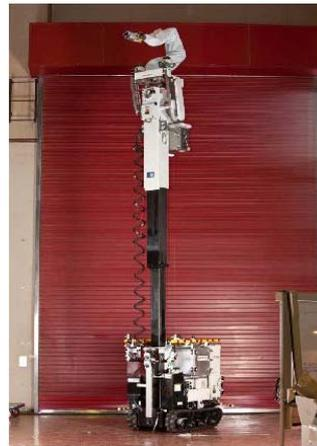
Inspection robot for high location
