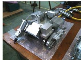
Inspection Robot for Lower part of S/C
