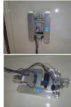
Robot for Measurement of S/C Water Level
