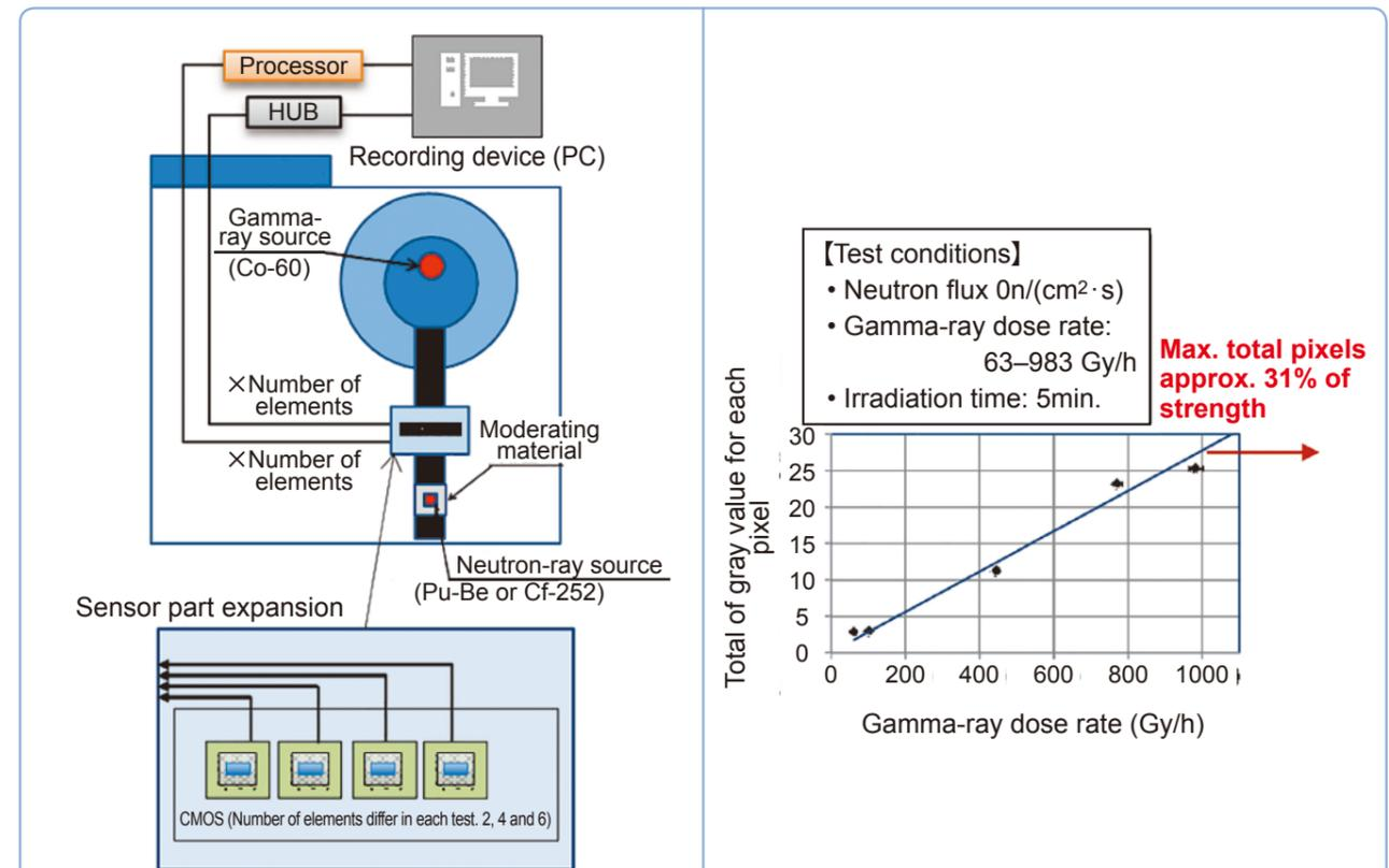
Fig. 1: Layout of Performance Validation Test
