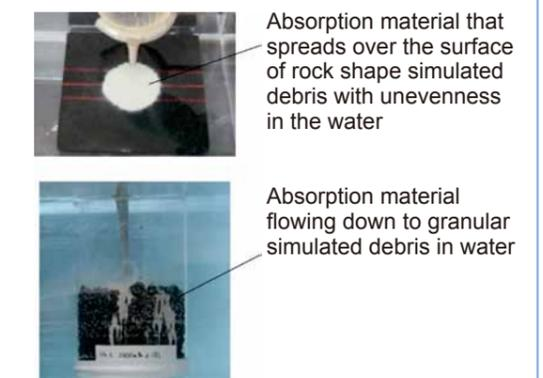
Fig. 6: Example of Workability Verification Test of Water Glass Type Absorption Material
