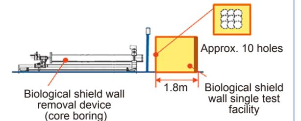
Fig. 4: Element Test of Biological Shield Wall Removal
