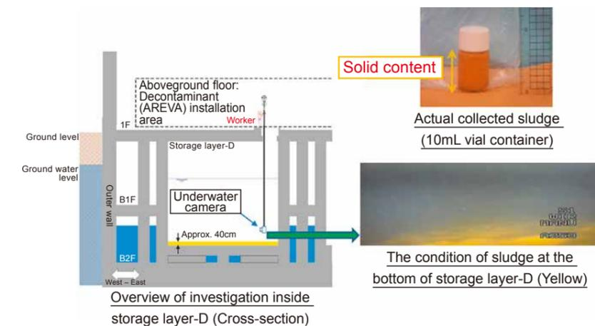
Fig. 4: Investigation inside Main Process Building Storage Layer-D and Collection of Sludge from Decontamination Device
