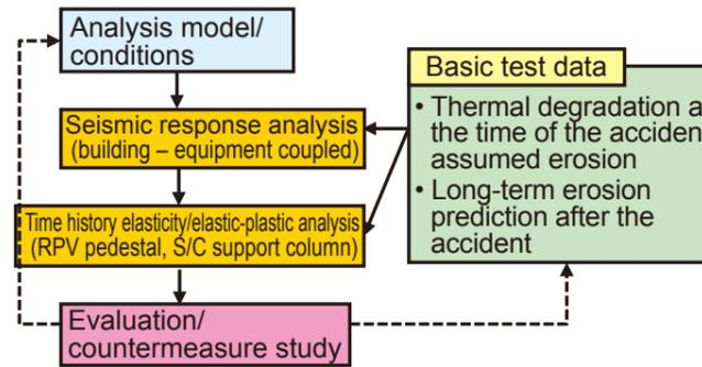
Fig. 1: Overall Development Flow of Seismic Analysis Method
