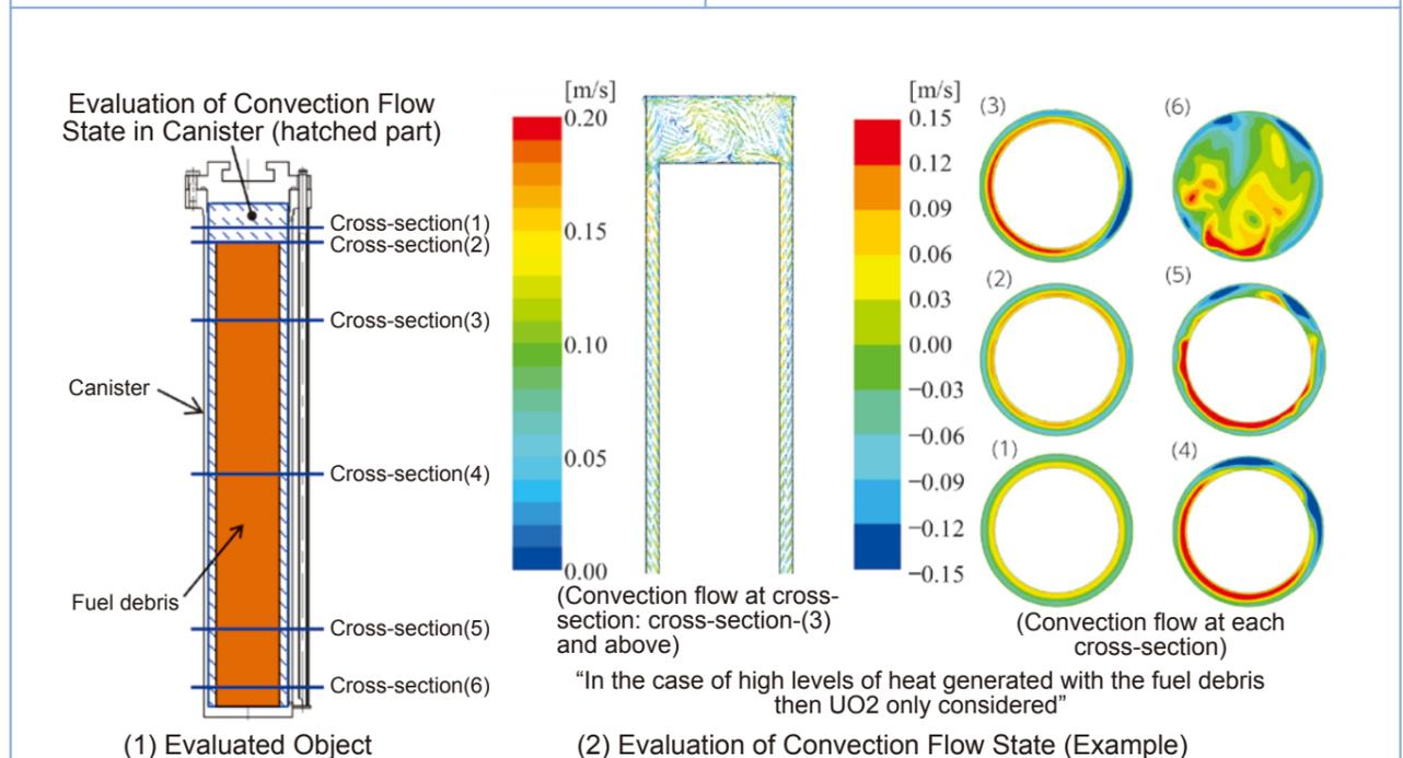
**Fig. 3: Evaluation of Convection Flow State in Canister**
