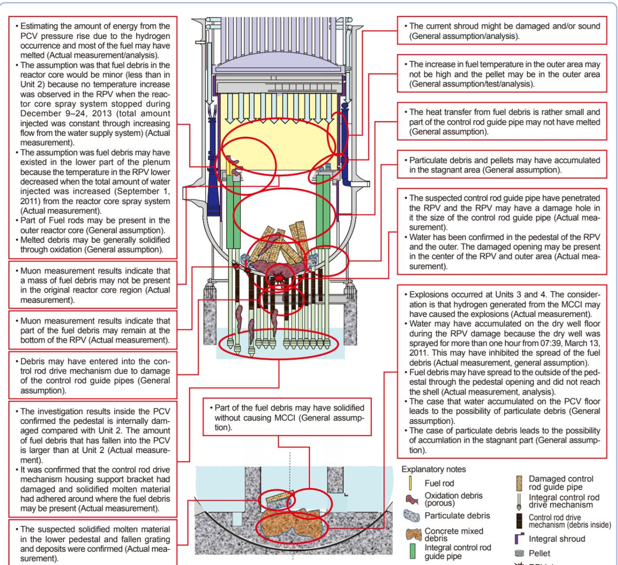
Fig. 1: Diagram of Estimated Fuel Debris Distribution (Example of Unit 3) As of February 28, 2018
