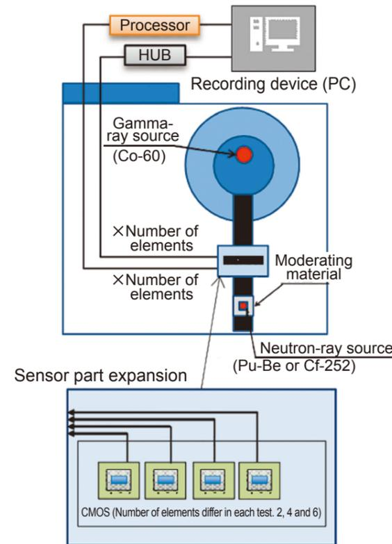
Fig. 1: Layout of Performance Validation Test
