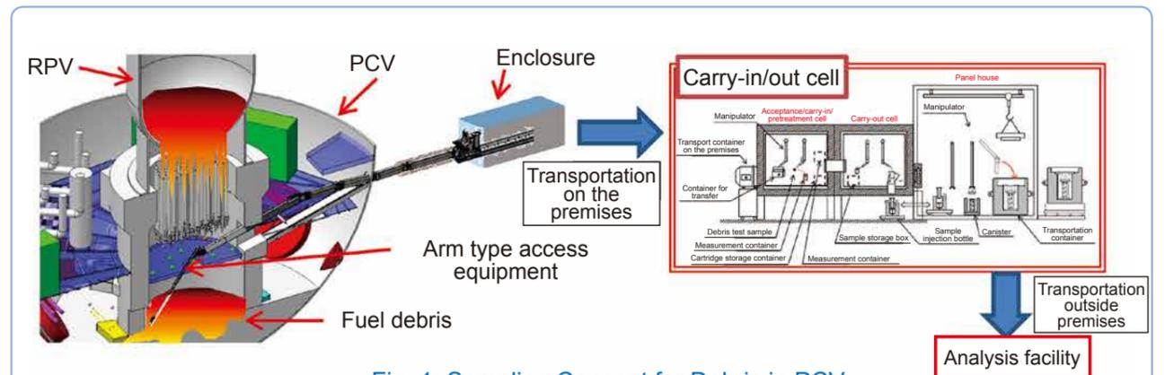
Fig. 1: Sampling Concept for Debris in PCV
