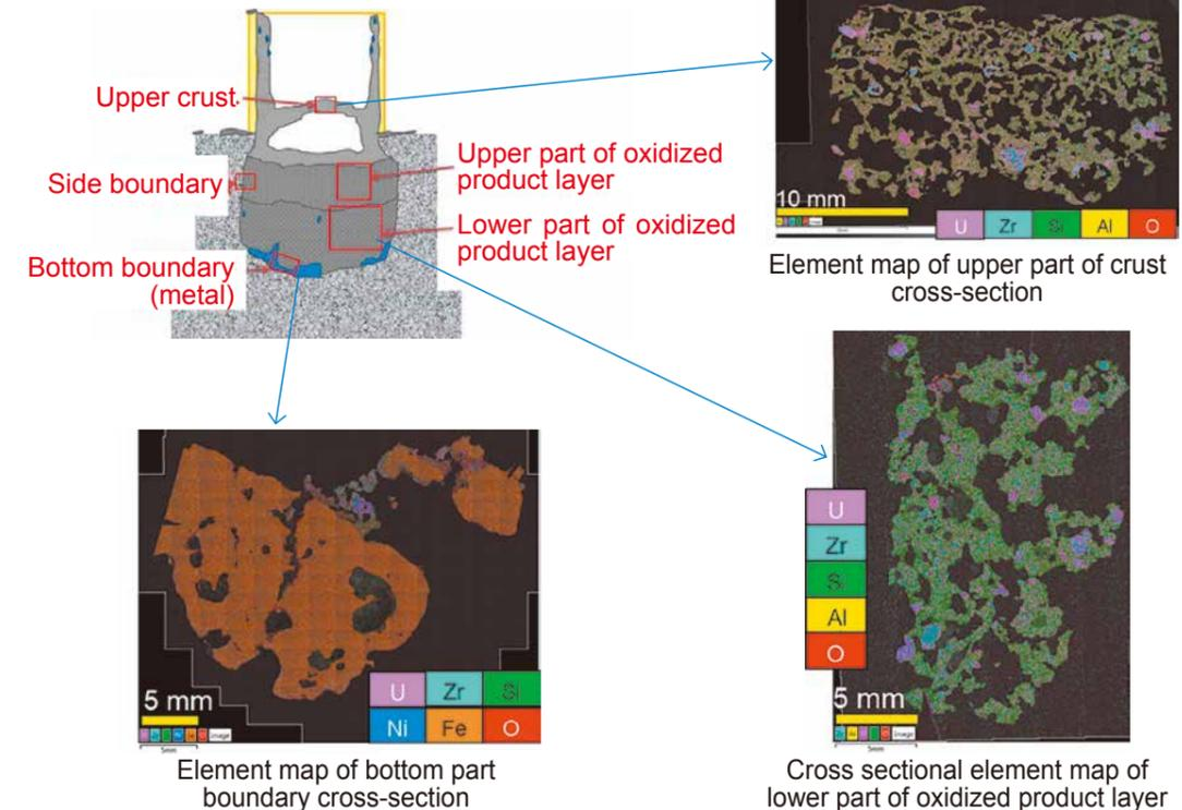
Fig. 1: Element Distribution of Large MCCI Test Products
