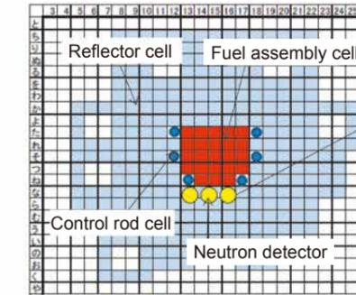
"Example Test Reactor Core"
