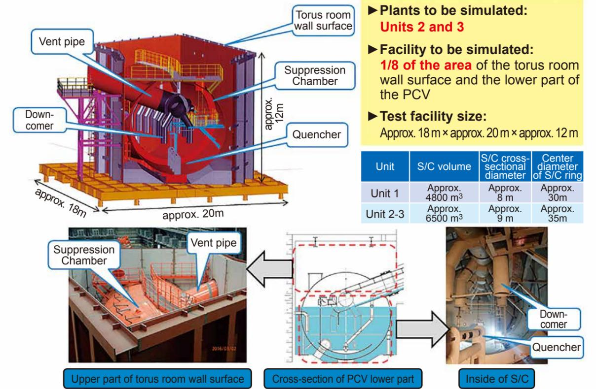
Fig. 1: Overview of Test Facility
