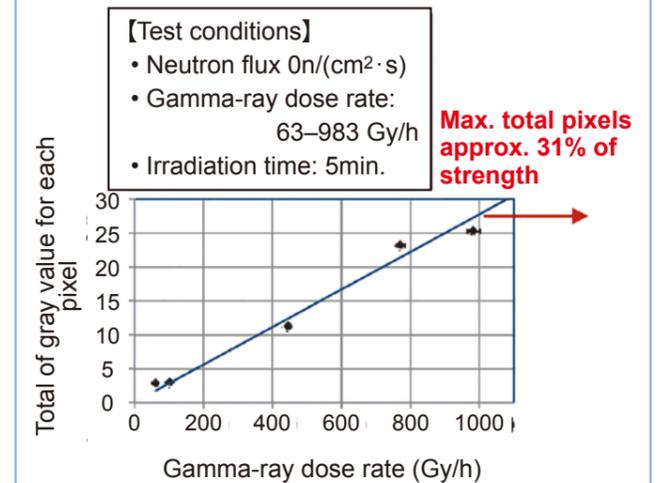
Fig. 2: Detection Performance at Single Gamma-ray Location
