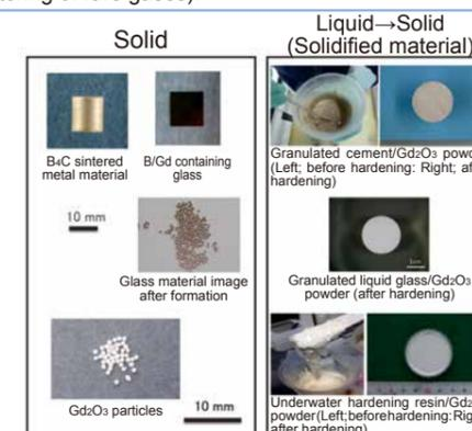
Fig. 5: Appearance of Insoluble Neutron Absorption Material (candidate material)
