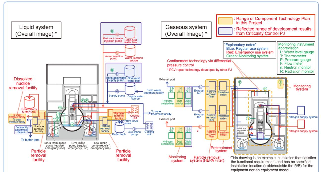
Fig. 1: Scope of Element Technology Development for System Formulation
