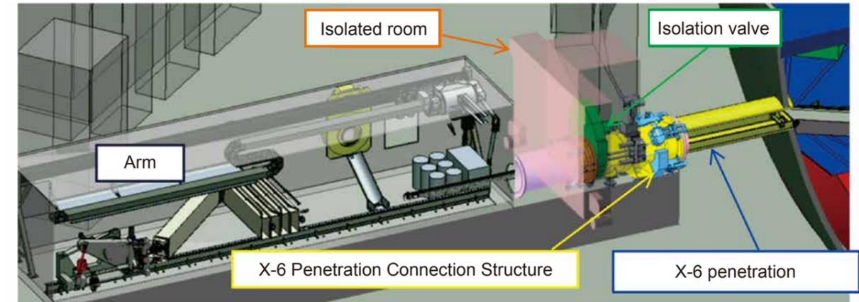
Fig. 1: X-6 Penetration Connection Structure
