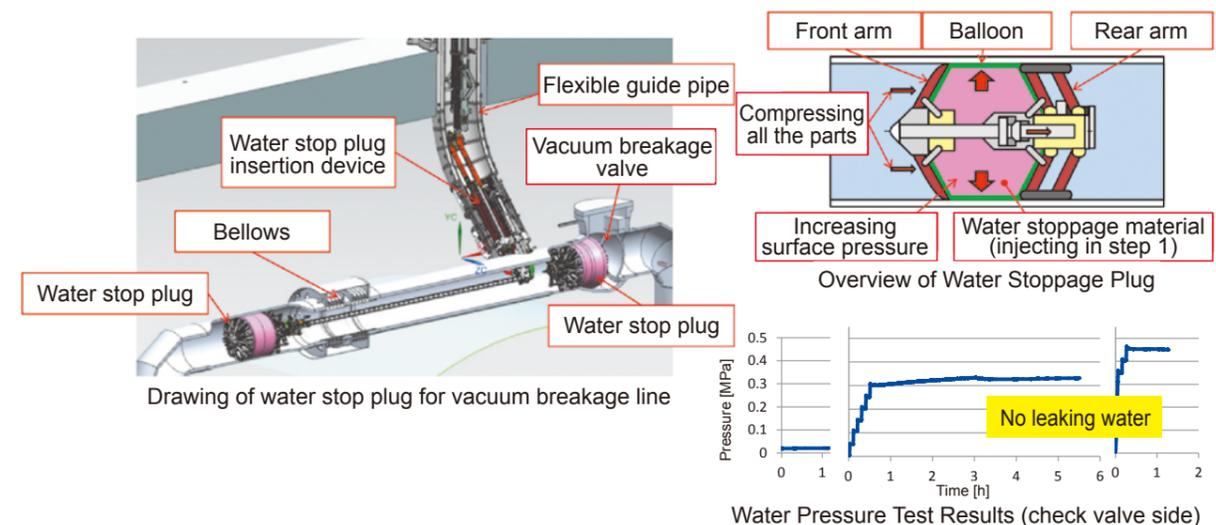
Fig. 2: Overview of Repair of Lower Part of PCV (Vacuum Breakage Line Filled)
