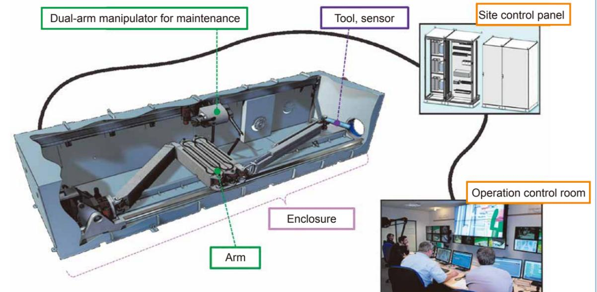
Fig. 3: Arm Type Access Unit
