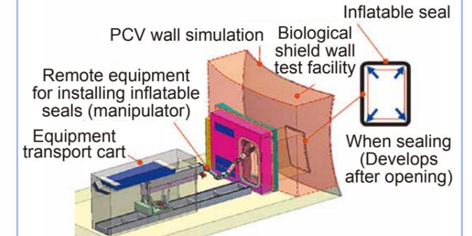
Fig. 2: Inflatable Seal Element Test
