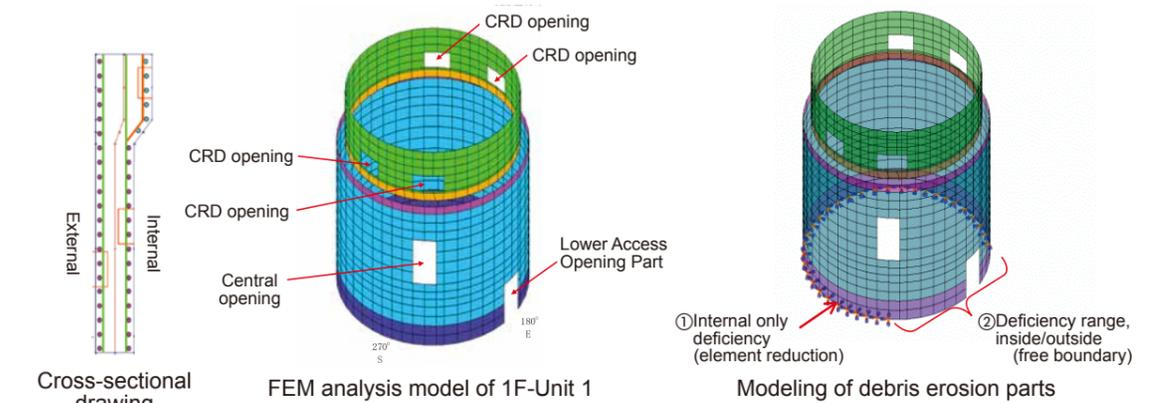
Fig. 5: Development of Seismic Evaluation Method for Pedestal due to Debris Erosion
