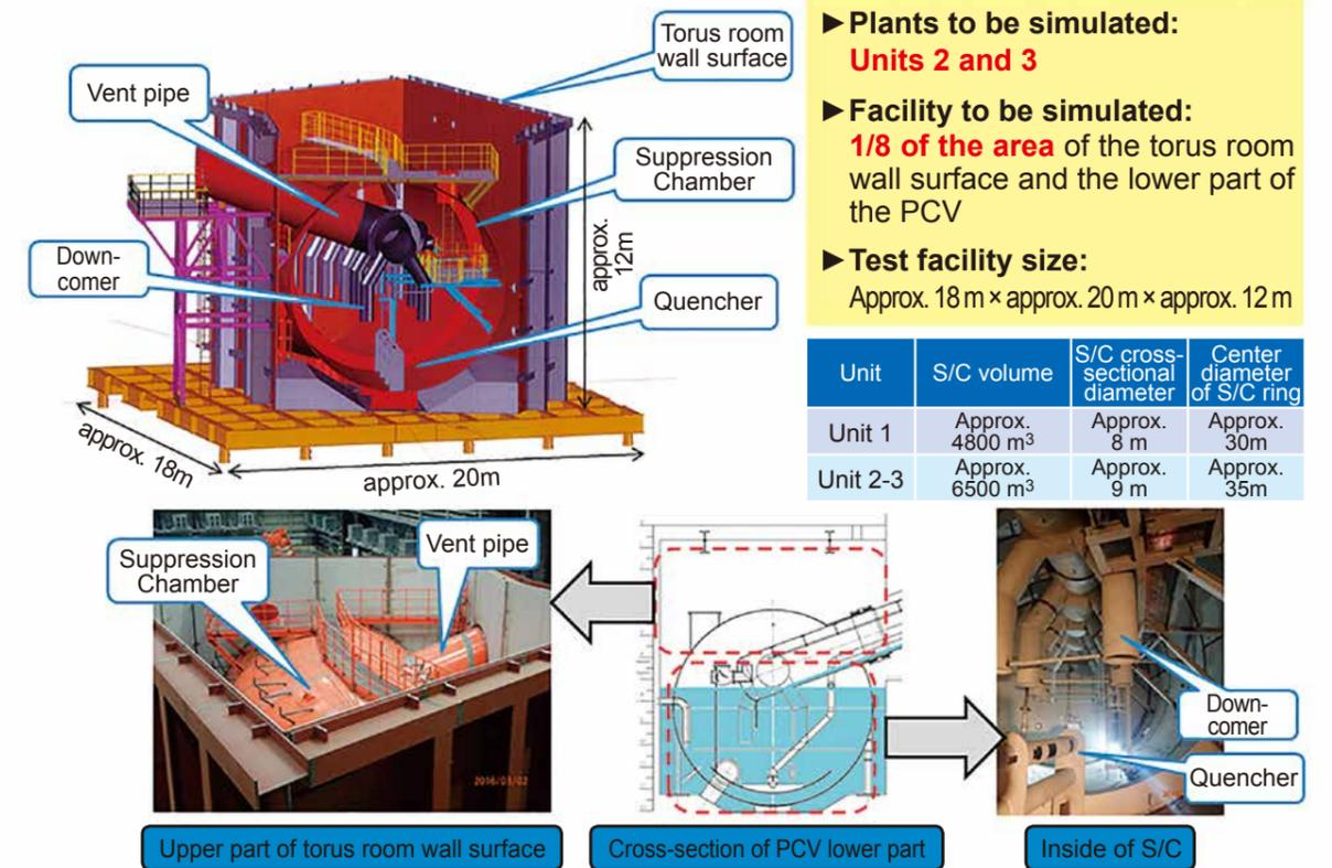
Fig. 1: Overview of Test Facility
