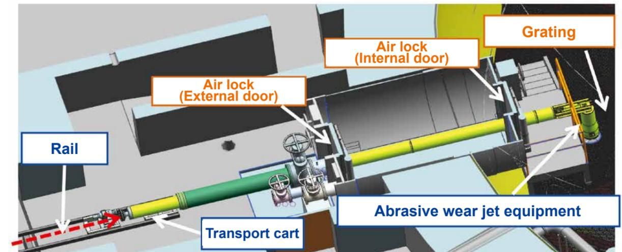
Fig. 2: Perforation Device for X-2 Penetration (Air Lock) Internal Door
