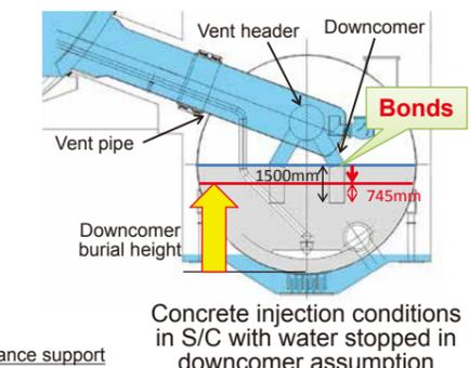
Fig. 3: Vent Pipe–S/C System Coupled Analysis Conditions and Time History Seismic Response Analysis Model (Unit 2–3)
