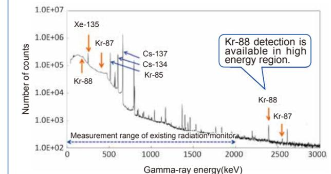
Fig. 4: Result of Gamma-Ray Measurement Tests by Gas Control System
