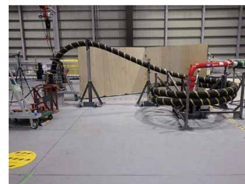
Photo-3: Supplying Water Stoppage Material for Injecting Filling to Stop Water inside S/C
