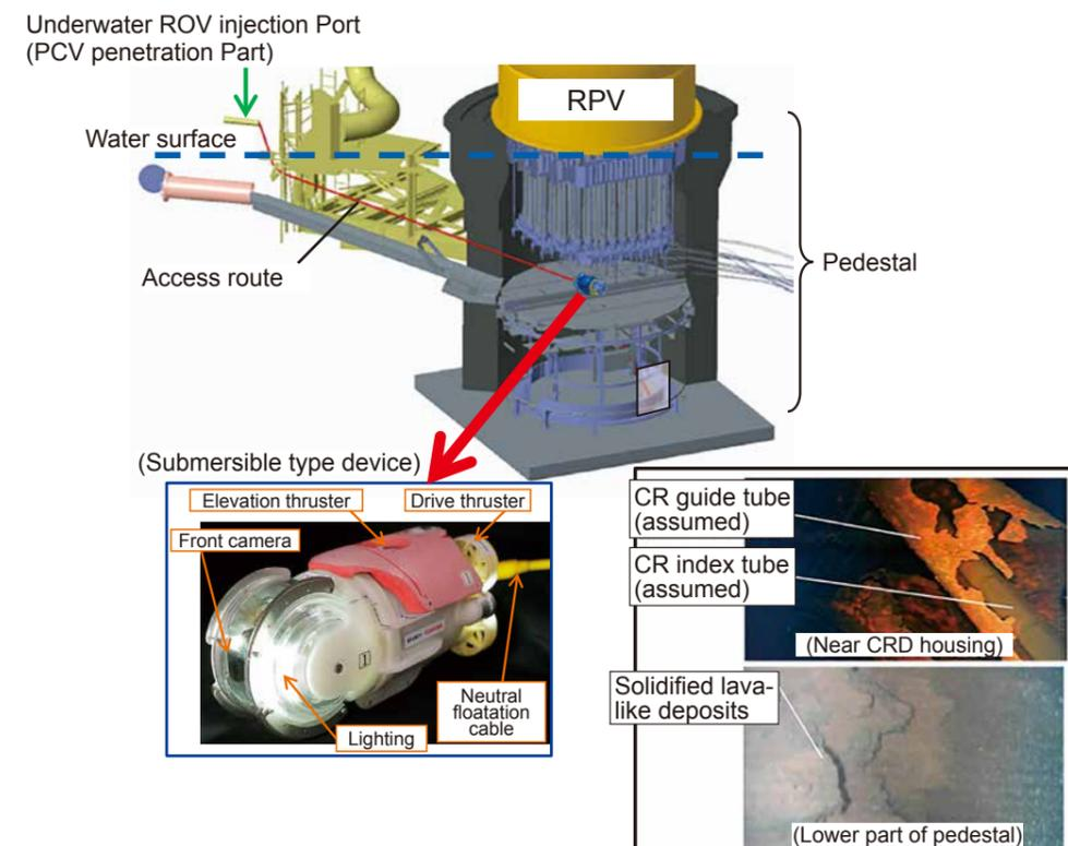
Fig. 2: Appearance of Submersible Type Device and Survey Route
