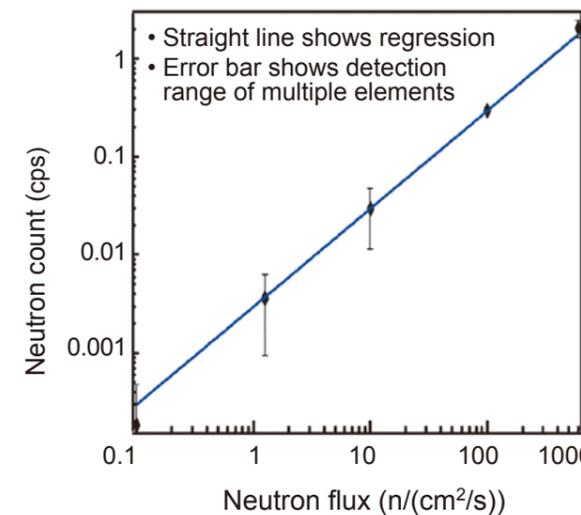
Fig. 3: Detection Performance with Single Neutron Location
