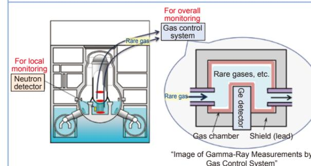
Fig. 3: Overview of Criticality Monitoring
