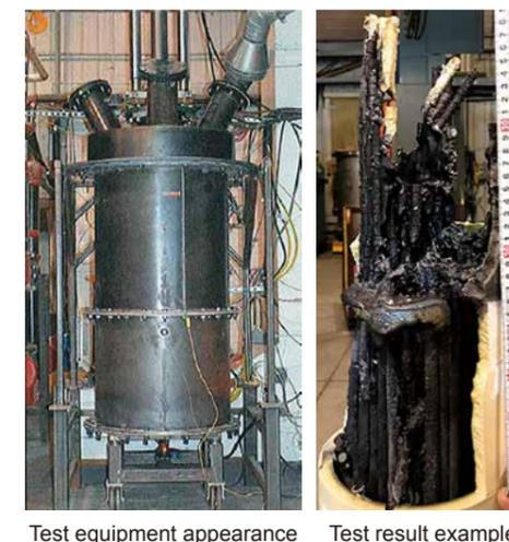
Fig. 2: Plasma Heating Test of Simulated Fuel Assemblies
