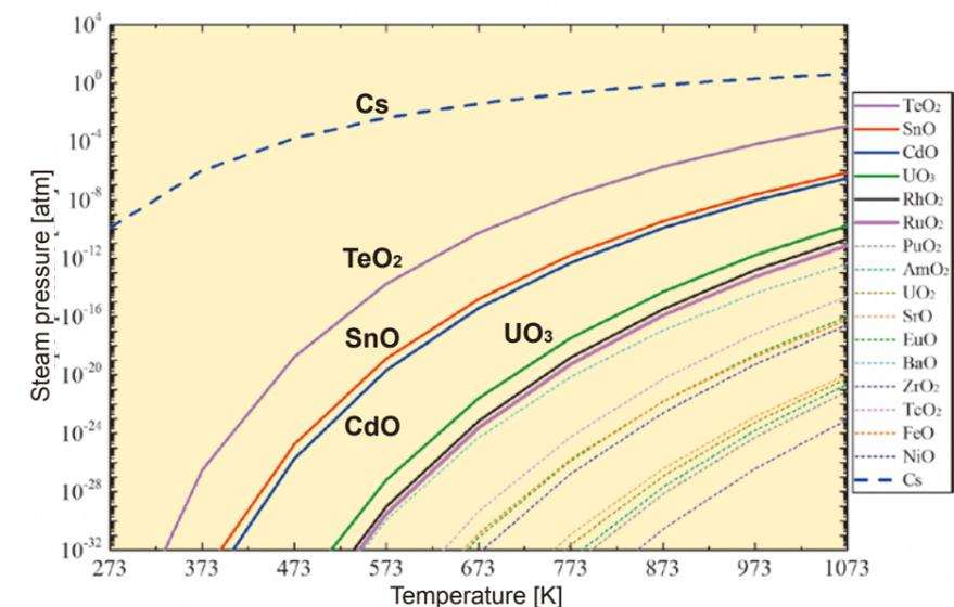
Fig. 2: Calculation Results of Steam Pressure of Oxidized Products
