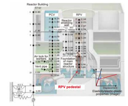
Fig. 2: Reactor Building/Large Equipment System Coupled Model
