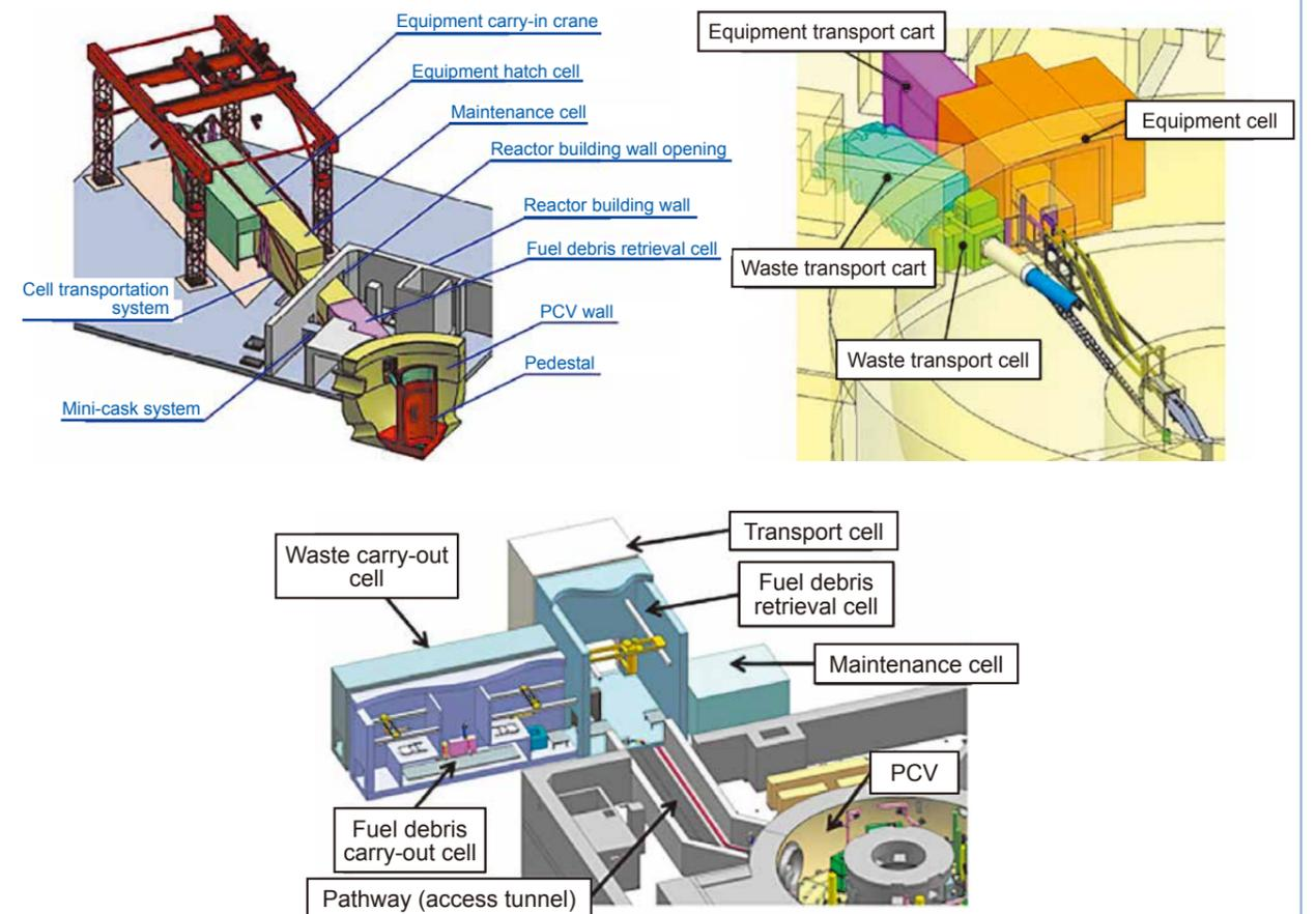
Fig. 2: Installation Image of Fuel Debris Retrieval Cell
