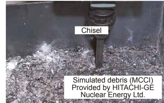
Fig. 1: State of Chisel Processing Preliminary Test
