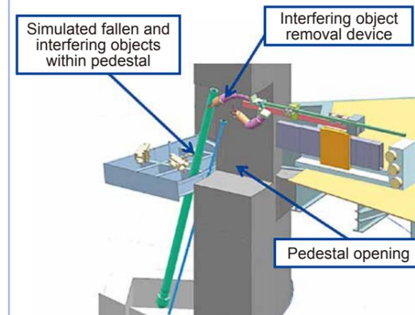
Fig. 3: Element Test of Removal of Interfering Objects in Pedestal
