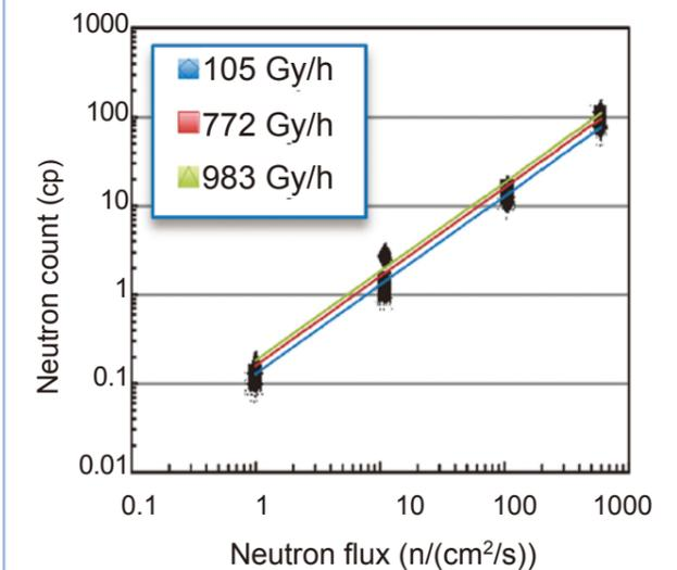
Fig. 4: Detection Performance with Gamma-Ray/ Neutron-Ray Combined Locations
