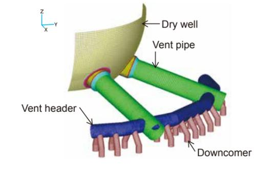
Fig. 4: Detailed Analysis Model of Vent Pipe for Elastic-Plastic Analysis and S/C System (Unit 2–3)
