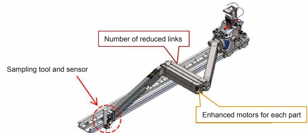
Fig. 2: Example of Access Device Used for Sampling
