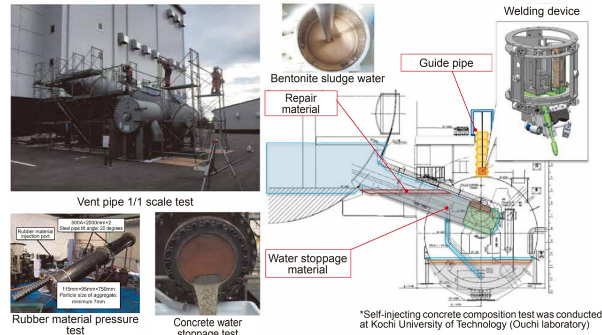
Fig. 1: Overview of Repair of Lower Part of PCV (Filling in Vent Pipe and S/C)
