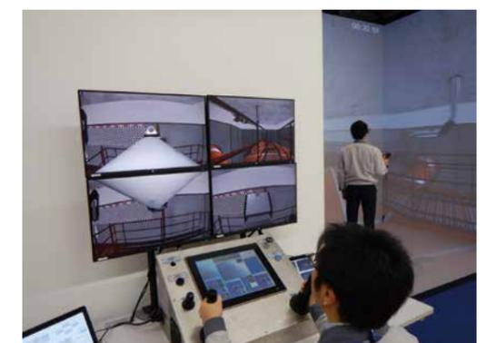
Photo-4: Operating Panel of VR System and 3D Screen
