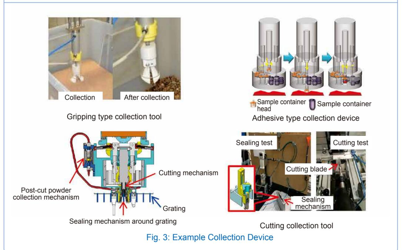
Fig. 3: Example Collection Device
