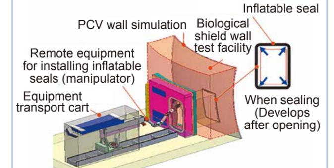
Fig. 2: Inflatable Seal Element Test
