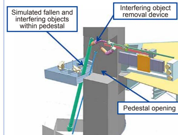
Fig. 3: Element Test of Removal of Interfering Objects in Pedestal
