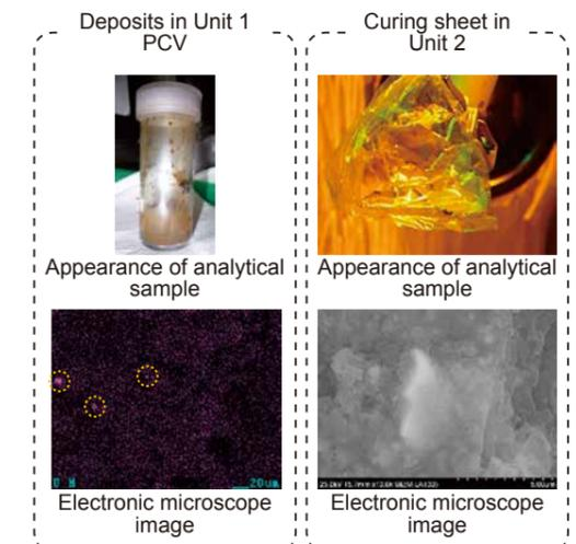
Fig. 3: Example of Analysis Sample and Analysis Results
