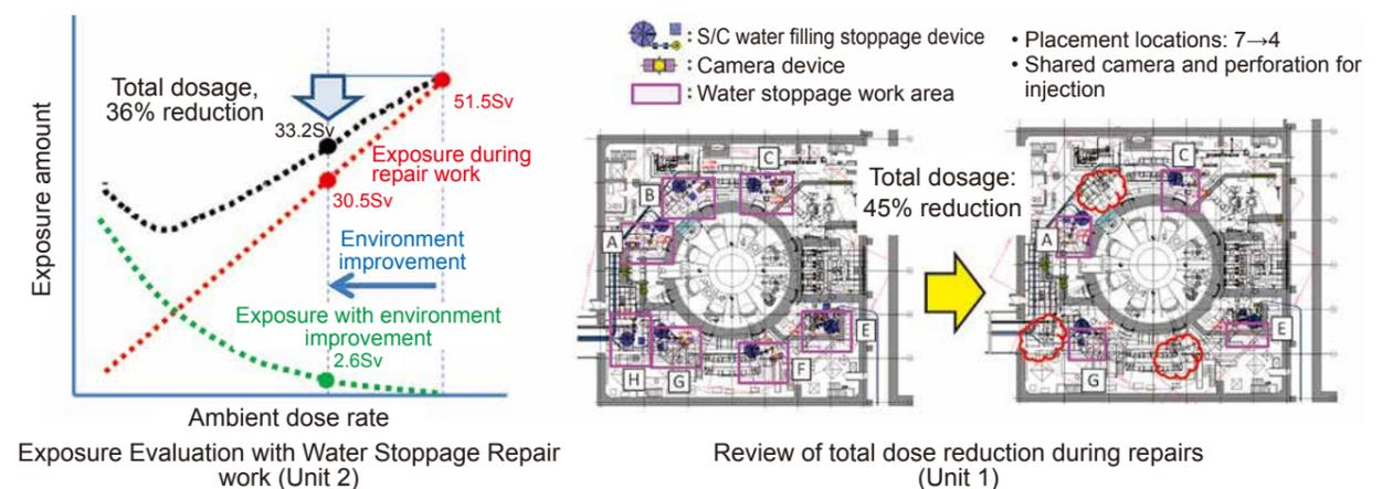
Fig. 3: Conceptual Study of Environment Improvement for the Applicable Repair Method (Example)
