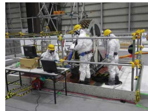
Photo-1: Implementation of S/C Support Column Reinforcement Test
