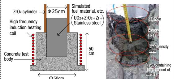
Large MCCI test apparatus in cooperation with CEA and its test product generated in MCCI test
