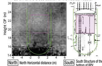
An image of high density substance thought to be fuel debris is confirmed on the bottom of the RPV. \*The measurement at unit 2 was conducted by TEPCO Holdings as a part of the IRID activities.
