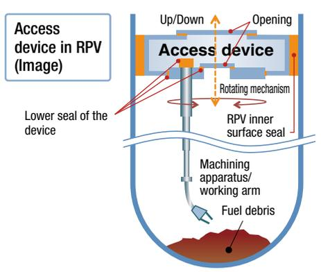
**AR Side access method: Access rail method** – Image of debris retrieval –
