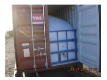
A PacTank within a standard 20' container can hold a maximum of 22.7m3 (6,000 gallons) of liquid. Other intermodal containers can also be used.
