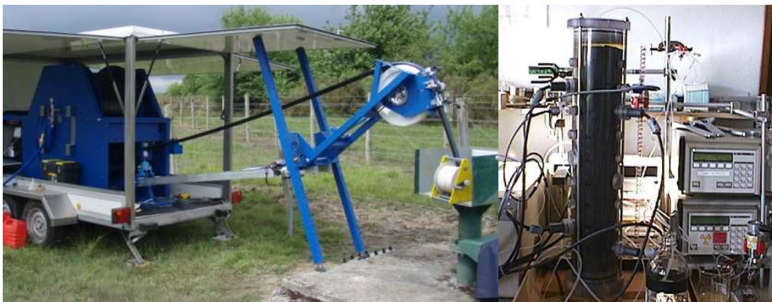
Trailer for pumping test up to 150 meter depth – Column experiment
