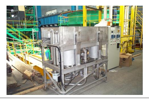
The SCRU can be moved around within the cooling pond using the existing skip handling equipment and placed in a convenient location. It operates under 6m (20ft) of water, utilising the pondwater for shielding. The SCRU module comprises a pump, a pre-filter to screen out particulates, two ion-exchange cartridges containing a Caesium-specific molecular sieve, and a post filter to prevent any potential release of resin into the pond environment.
