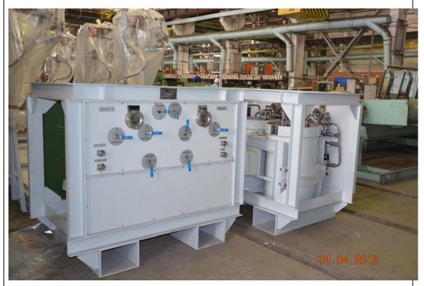
The figure pictures two assembled filter-container units ready for shipment to a Russian radiochemical enterprise where the LWR processing is under way.
