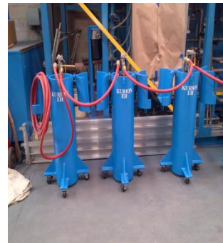
Kurion Modular Cs Removal Vessels (EH), Sr Removal (TS-G) and Full, Shielded, Lead-Lag Modular System
