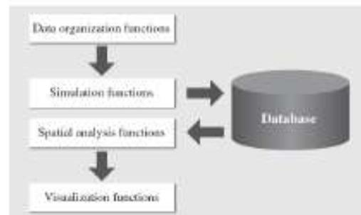
Fig. 8. System Functions and Flow. This figure shows each function and a system flow chart. The data organization and simulation functions make use of water resource cycle simulation technologies, and the spatial analysis and visualization functions make use of visualization technologies based on the geospatial information system (GIS).
