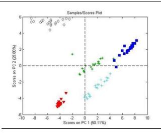
Example of discrimination of steel samples using chemometrical data treatment
