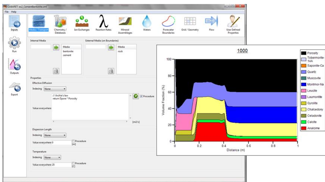
Figure 1: CABARET GUI showing part of the input for a simulated reaction between cement, bentonite and porewater and a plot of simulated mineral assemblages across the cement across the cement-bentonite boundary (at the left margin of the plot), produced using graphing software bundled with CABARET.
