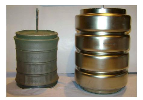
The design of the HIP can will require that contaminated water can pass freely into and out of the HIP can. This would be achieved in service by having filters built into the end caps. After the
