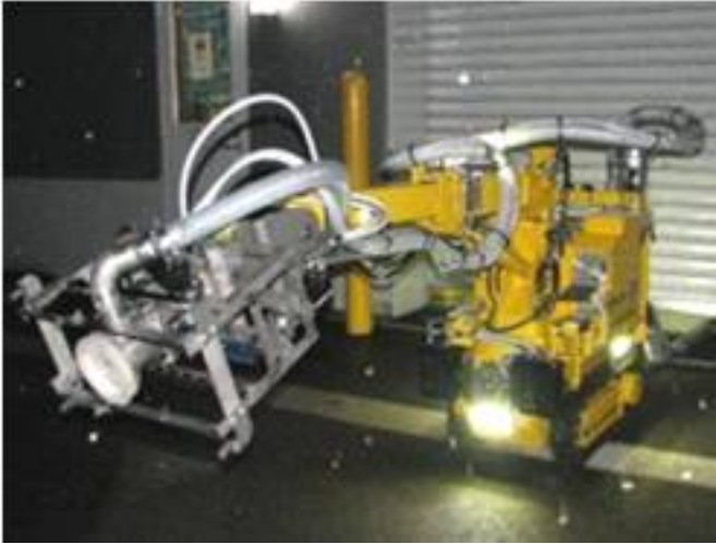
High-pressure water jet decontamination device
