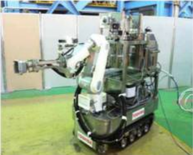
Dry ice blast decontamination device
