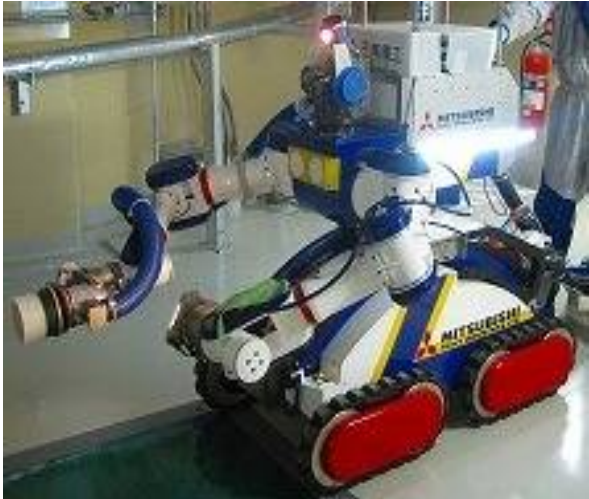
Blasting/collecting decontamination device
