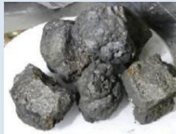
UO<sub>2</sub>\_In-vessel試料 (No. 6) の外観
