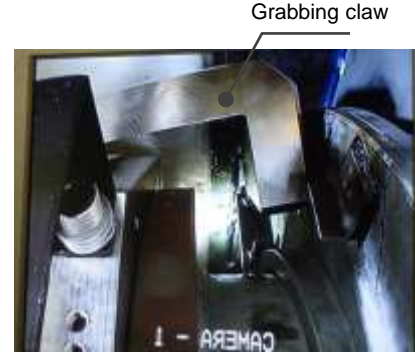
③ Grabbing and connection to the X-6 penetration
