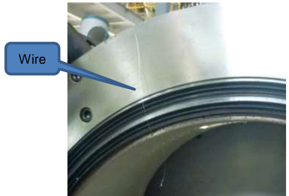
Verification of impact of foreign objects on airtightness
