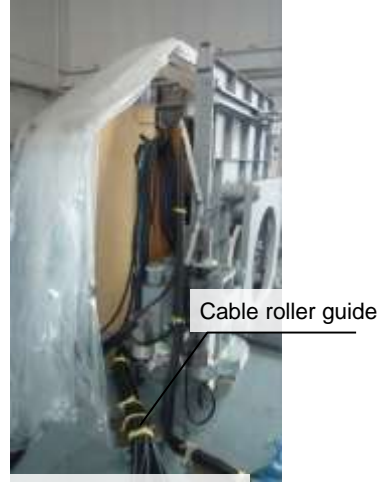
Cable after installation (cable management)
