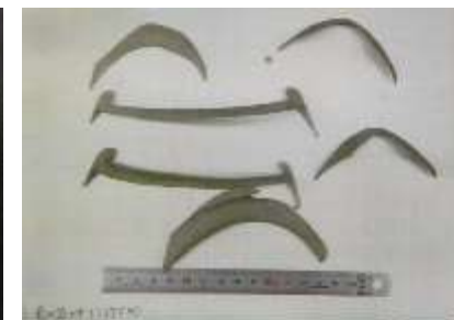
Falling cutting scraps found inside the steam separator (example)
