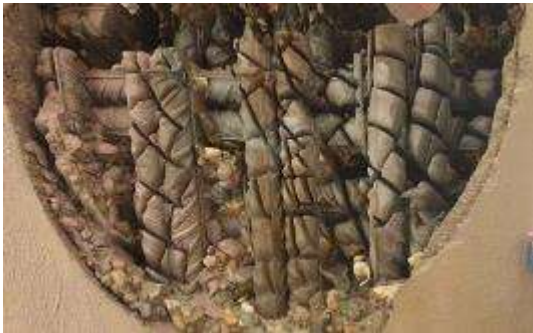
Cutting the main rebars of the biological shielding wall in the element test
