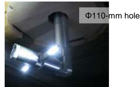
Investigation equipment B2 with its pan/tilt mechanism activated and stretchable light arms fully extended after passing through the hole in the shroud head
