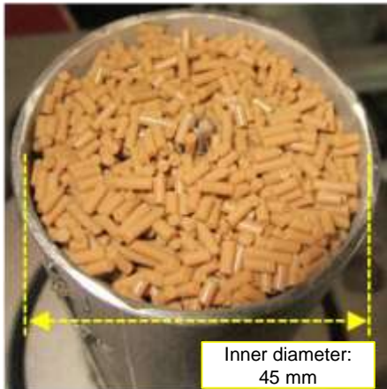
Figure: External appearance of a test container filled with water containing particle samples
