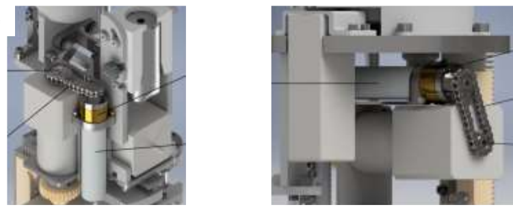
Adding a recovery motor in case of main motor failure
