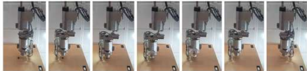
Fuel debris collecting test
