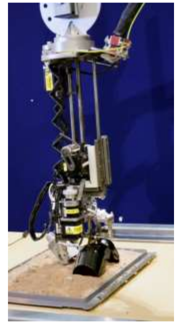
Fuel debris collecting test
