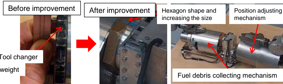
Connection test for debris collecting and position adjusting mechanism
