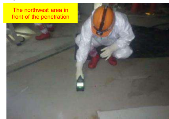
Detecting buried metal in the reactor building
