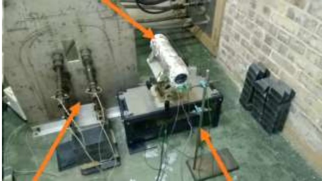
Radiation Sources Appearance of calibration facility Ambient Temperature Thermocouple (near)
