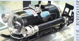
[Scope of investigation] Equipment drifts through the water in the torus room up to the submerged sand cushion drain pipe outlet to detect leaks of 1 L/min or more from the submerged sand cushion drain pipe outlet using lights, camera, and a tracer
