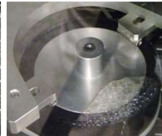
Verification of leakage in the controlled inclination type seal under 0Gy (unirradiated) and 50°C conditions
