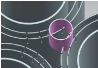
Conceptual image of cutting the steam separator (Hole saw)
