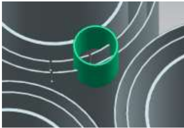
Conceptual image of cutting the steam separator (Hole saw)
