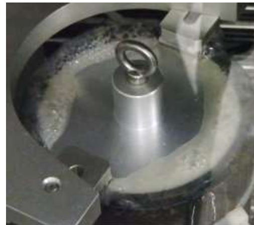
Verification of leakage in the regular seal under 0Gy (unirradiated) and 50°C conditions
