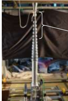
The stage on the tip side does not retract completely
