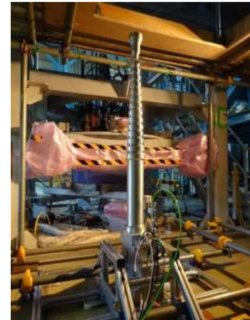
Element test for the 14-stage telescopic guide pipe
