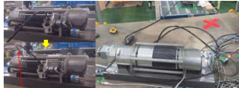
Cable is fed to the rear of the drum
