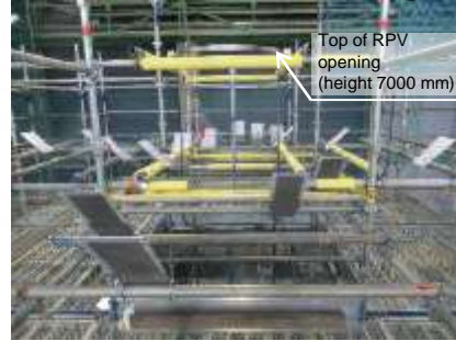
RPV interior (investigation area) simulation
