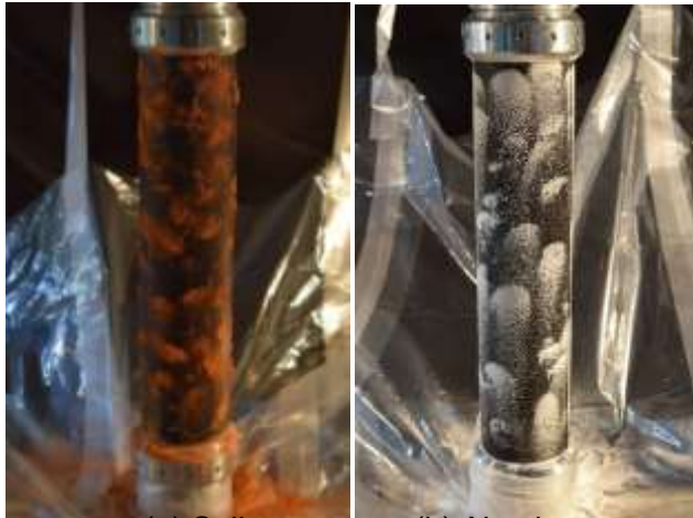
(a) Soil Powder adhered to the entire outer surface of the pipe (b) Alumina
