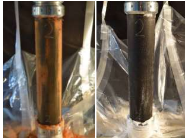
(a) Soil There are wiping streaks Condition of pipe outer surface after retraction and re-extension (b) Alumina
