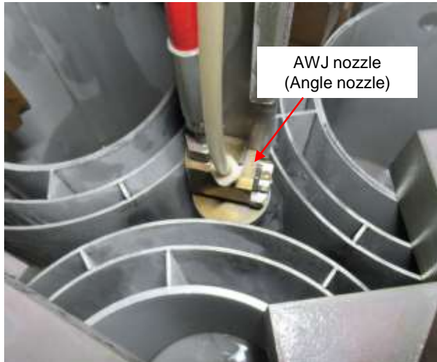
Photo ① of test pieces before cutting
