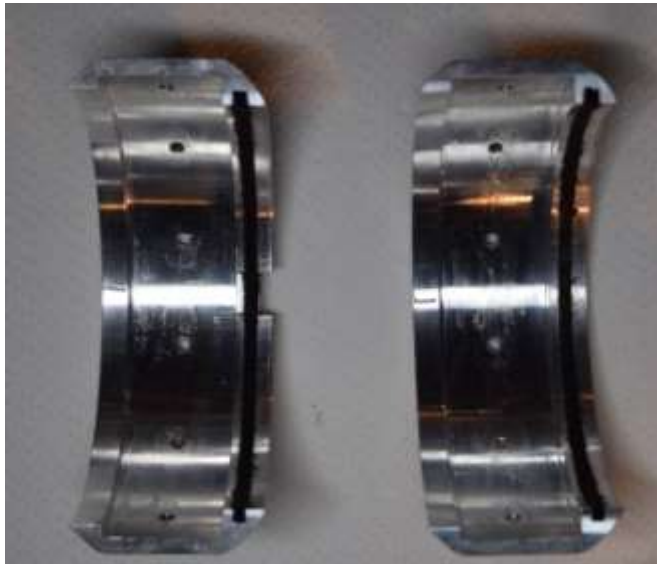
Appearance of scraper at the tip of the 1st stage pipe after pressure resistance test (disassembled state)
