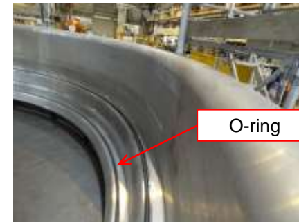
O-ring for the container (Sealed part [6] dovetail groove)
