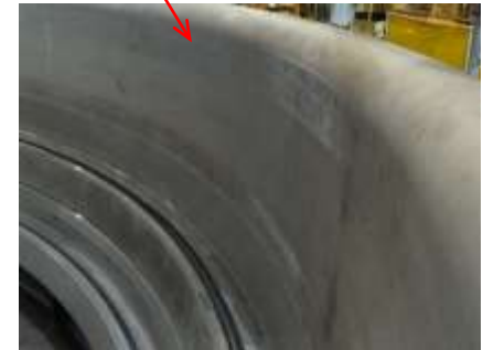
Inner surface of the movable flange (after the test)
