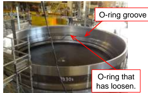
O-ring for the movable flange (Sealed part [3] U groove)
