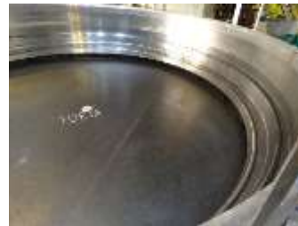
Movable flange, inner surface of container (After the test)
