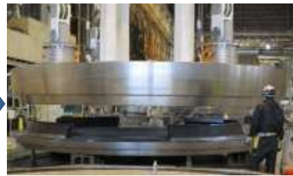
[2] Upper and lower lid fitting preparation
