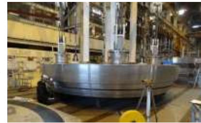
[3] Upper and lower lid fitting completion
