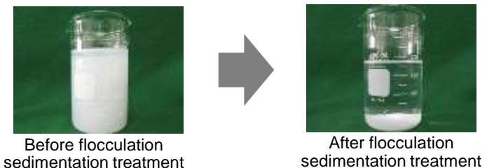
Figure RO-concentrated water treatment element test
