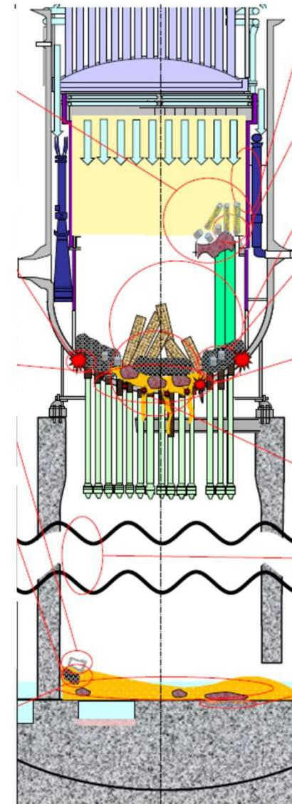
Damage estimation of the Unit 2 RPV/PCV
