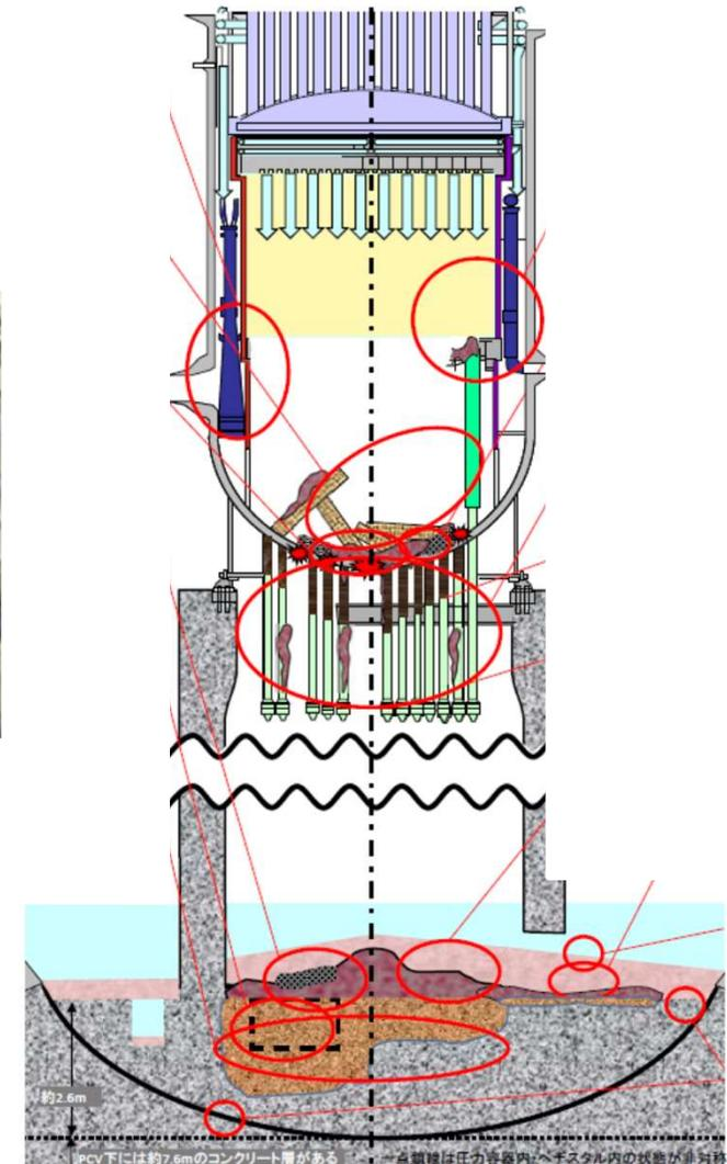
Damage estimation of the Unit 1 RPV/PCV
