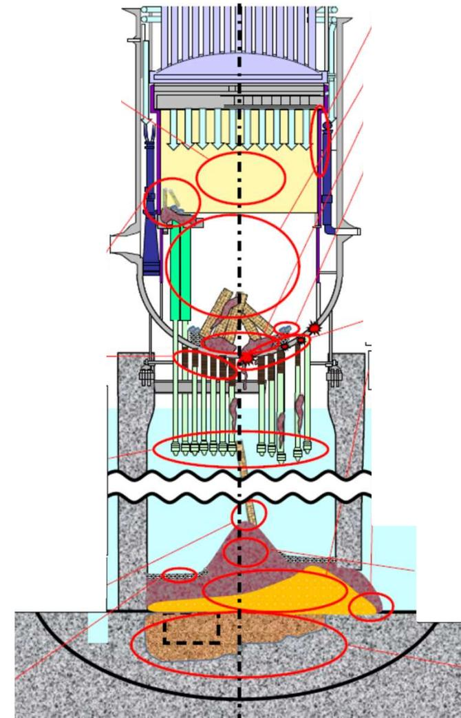
Damage estimation of the Unit 3 RPV/PCV
