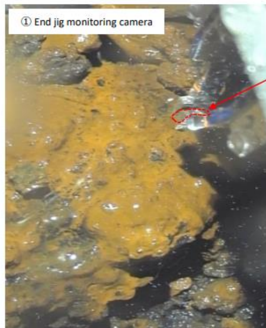
Grasping fuel debris below the opening 2
