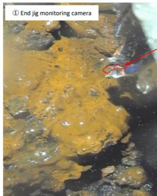
Grasping fuel debris below the opening 2
